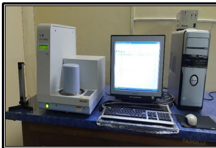
Figure 3.13 SII EXSTAR 6000 DSC model.
