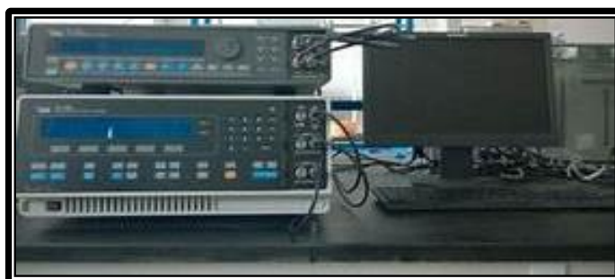
Figure 3.22 Solartron 1287 electrochemical interface with 1260 impedance gain phase analyzer.
