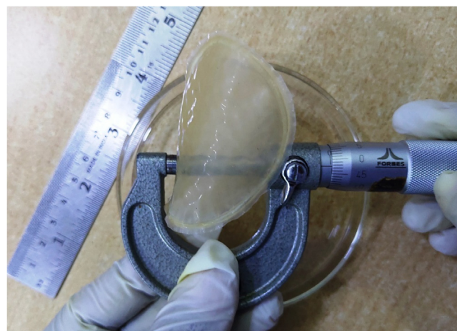
Fig. 1. A plasticized polymer electrolyte specimen \text{MgTf}_2/\text{PC-DEC}/\text{PEO} with 1 wt% MgO.
