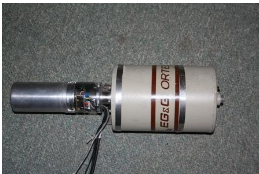
Figure 2.6: ORTEC GMX (Model number: GMX 20-70-5) HPGe detector
