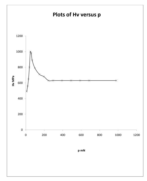
Figure –5 Plots of  $H_v$  versus p for  $Bi_{1.80}Sb_{0.2}Te_3$  crystal
