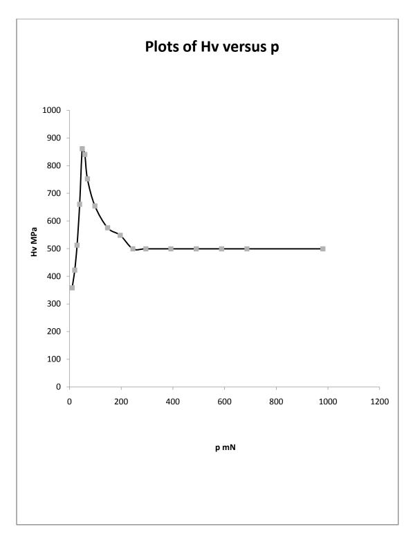
Figure –3 Plots of  $H_v$  versus p for  $Bi_{1.95}Sb_{0.05}Te_3$  crystal
