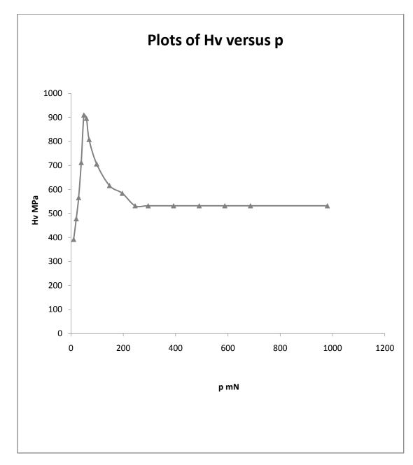
Figure –4 Plots of  $H_v$  versus p for  $Bi_{1.90}Sb_{0.1}Te_3$  crystal
