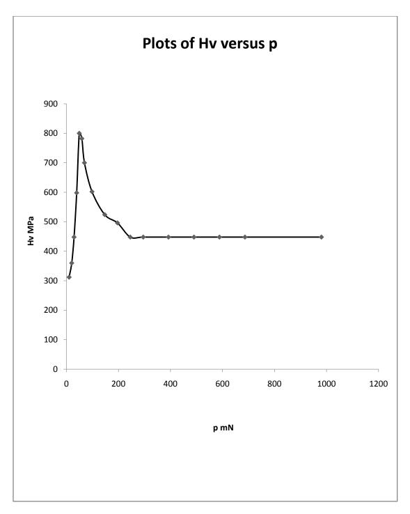
Figure –2 Plots of  $H_v$  versus p for  $Bi_2Te_3$  crystals
