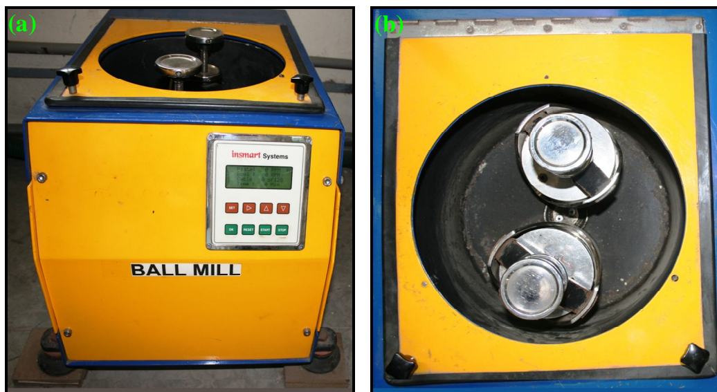
Fig. 3.2: Photographs showing planetary ball mill: (a) Front view and (b) Top view
