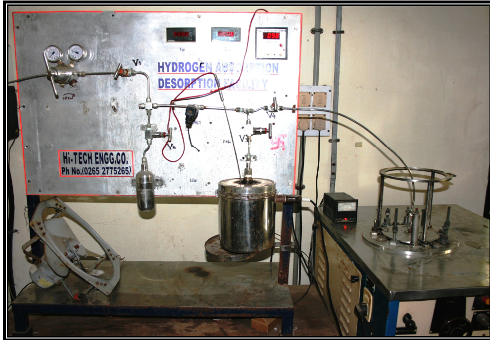
Fig. 3.9: Photograph showing experimental setup of hydrogen absorption and desorption apparatus
