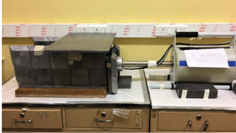
Figure 3.6: Pictorial view of typical source-detector counting setup at 14 UD Pelletron facility
