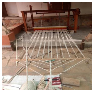
Plate 4.6n: The traditional pit loom which has now been replaced by the frame looms for weaving shawls at Khamir Organization (Reviving crafts), Kukma.
