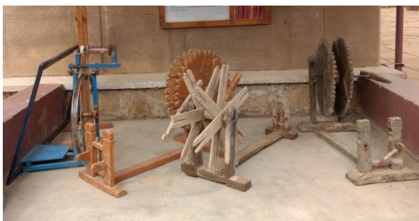
Plate 4.6g: The craftsmen uses the charkha or the spinning wheel used for spinning yarn from the woollen fibers.
