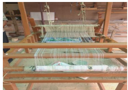
Plate 4.6n: The traditional pit loom which has now been replaced by the frame looms for weaving shawls at Khamir Organization (Reviving crafts), Kukma.
