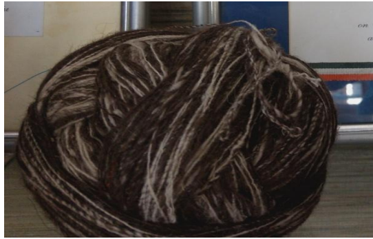
Plate 4.4g: Space dyed wool: An example of the space dyeing wool yarn. It was done 2-3 times. When woven it gave a different natural look to the shawl.
