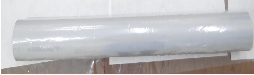
Plate 4.57: The poly vinyl chloride (PVC) pipe was first covered with the mylar and then covered with acid-free tissue over mylar.
