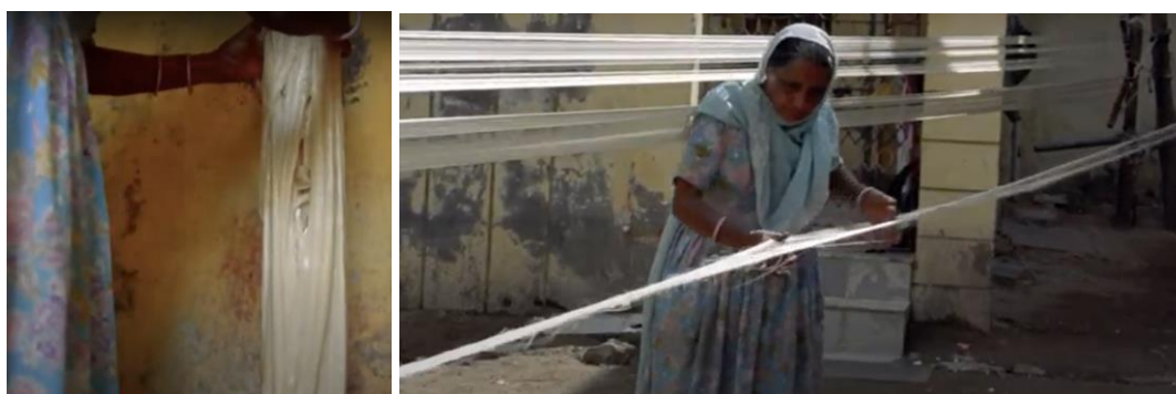
Plate 4.18: Application of starch on Tani & its stretch in open between poles
