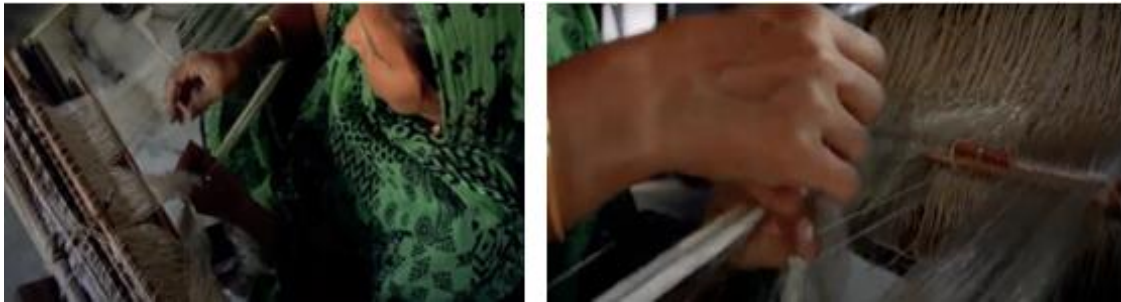
Plate 4.31: Joining of warp ends to Rach ends ( Sandhani )
