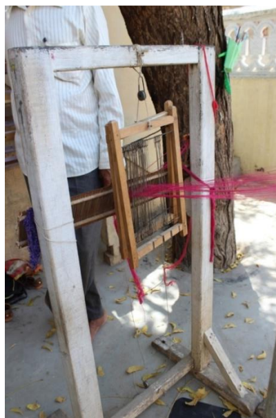
Plate 4.11: Yarns passing through alternate heddle & then through reed
