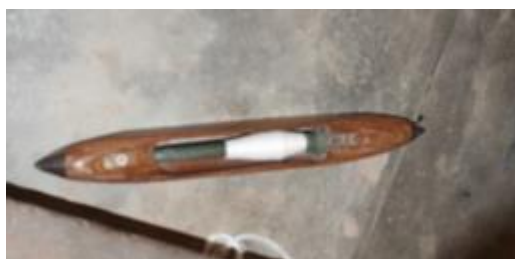
Plate 4.30: Shuttle filled with weft yarn
