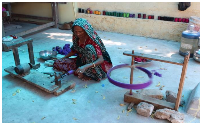
Plate 4.26: Electronic bobbin winding machine for weft yarn, in weaver’s workshop at Don
