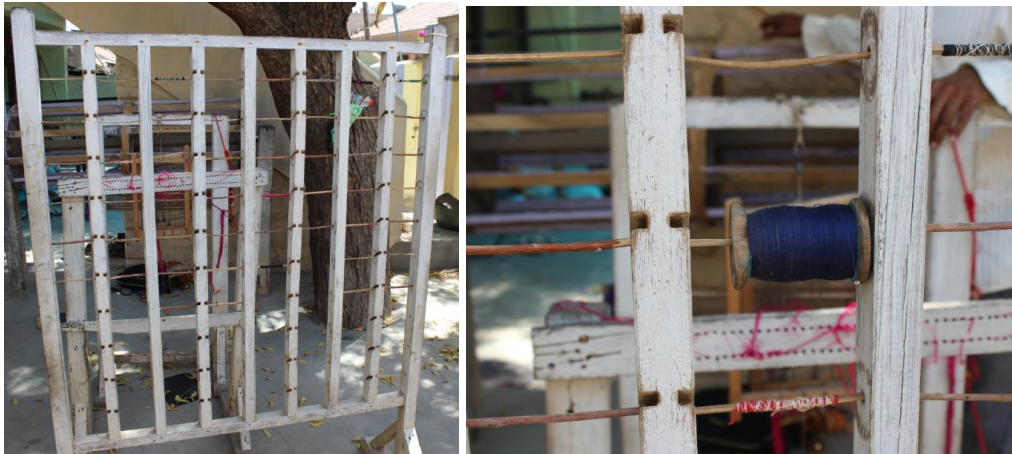
Plate 4.9: Traditional Wooden vertical crill – to hold yarn spools
