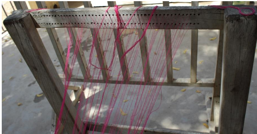
Plate 4.10: Yarns passed through the fixed heddle in vertical frame in alternate
