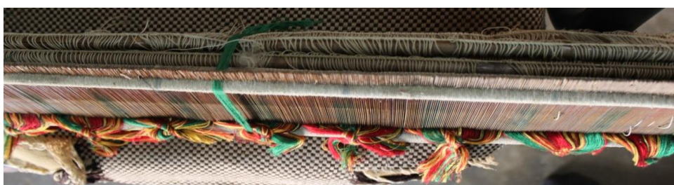
Plate 4.23: Fani with warp yarn as per fabric pattern
