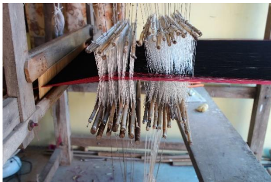
Plate 4.35: Multiple harnesses used in Mashru loom
