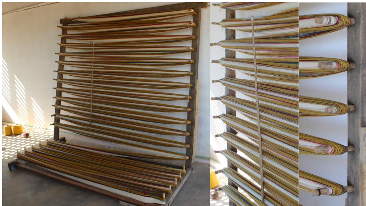
Plate 4.15: Detailed view of wooden warping frame and pegs
