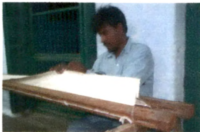
Plate-97: Holding the Markeen together using a hem-stitch
