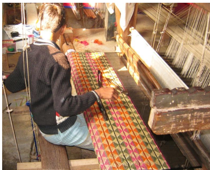
Phekwa technique (shuttle carrying weft across the width)
