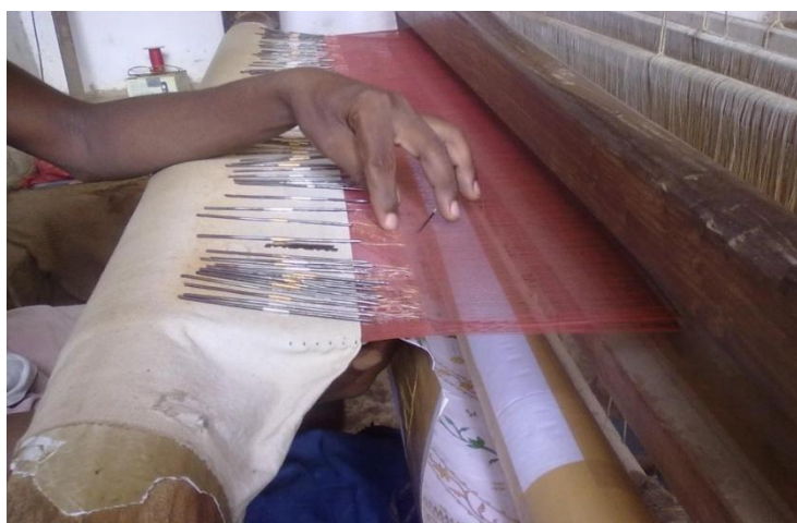
Karua technique (Graph kept under the warping before weaving)
