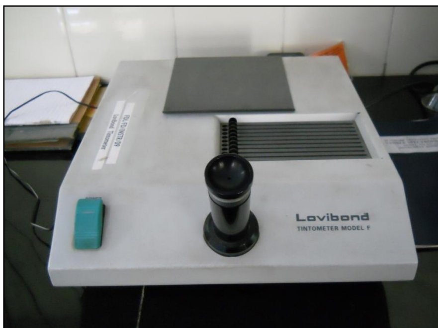
Plate 4.3.4.2.2: Lovibond tintometer for estimation of color of oil used for frying french fries and bhajias
