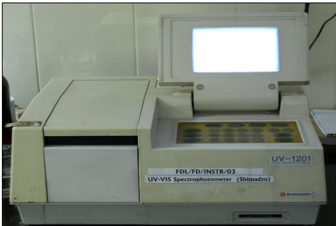
Plate 4.3.4.1.4.3.2: Shimadzu UV-1201 used for determination of p-anisidine value
