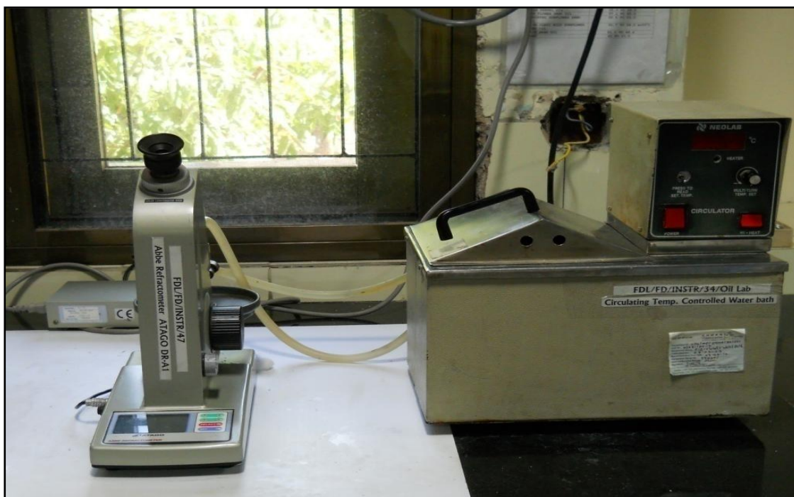
Plate 4.3.4.2.1: Abbe refractometer used for determination of refractive index of oil
