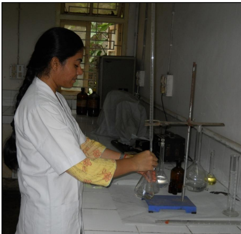
Plate 4.3.4.1.3.3: Determination of peroxide value by titration method
