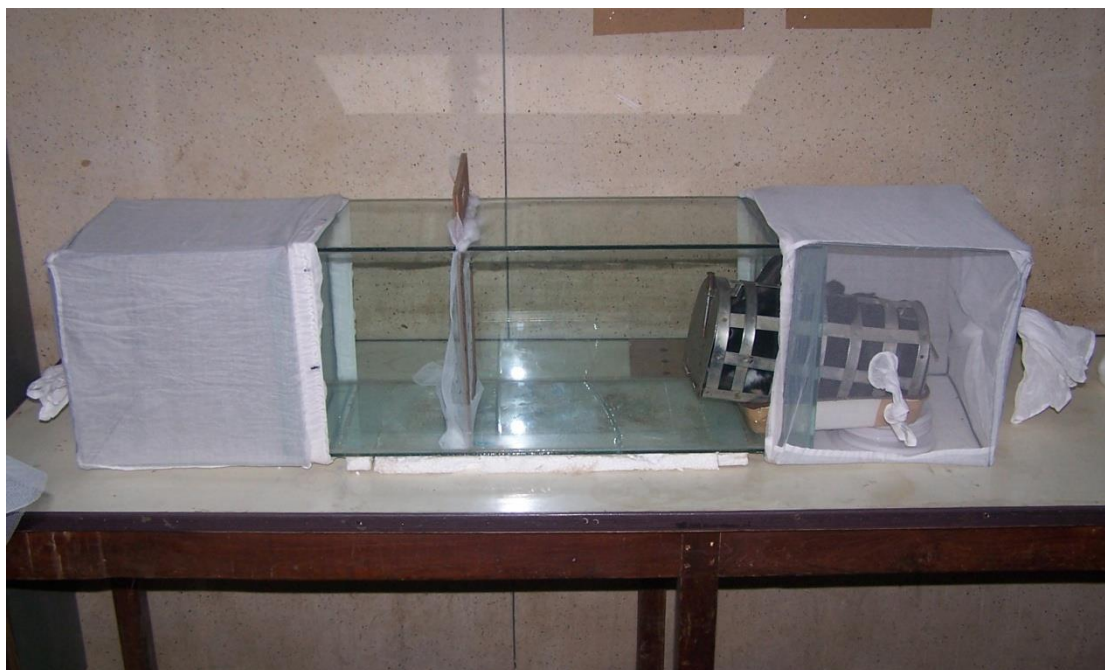
Figure 3A.10. Tunnel test assembly with rabbit at one end
