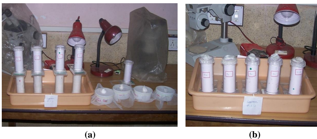
Figure 3A.13. (a) Exposure of mosquitoes on impregnated paper; (b) Exposure of mosquito on non-impregnated paper
