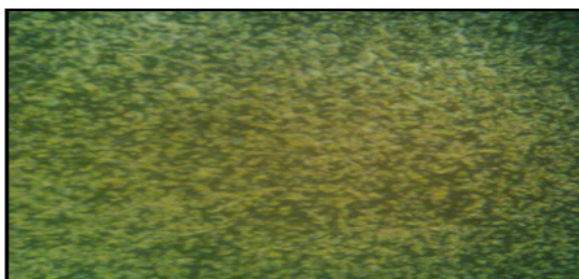
(e) Threaded texture of nematic phase
