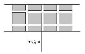
Figure 6.3 Capillary fissures model of porous matrix suggested by Irmay.
