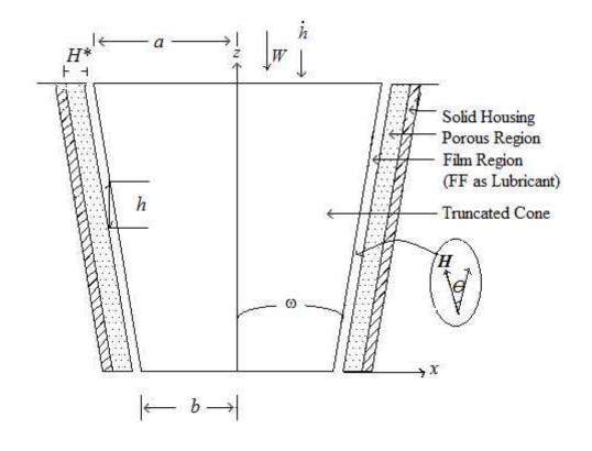
Figure 6.1 Schematic diagram of porous truncated cone squeeze film geometry.
