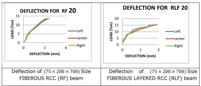
From the graphs of Load vs Deflection it is observed that, during the first elastic stage the curve is almost linear line. After yielding of beam the curve changed its slope and it became more flat. There was a considerable deviation in load deflection curve after the yielding of beam, which occurs first cracking and yielding of beam which caused a sudden increase in deflection.
