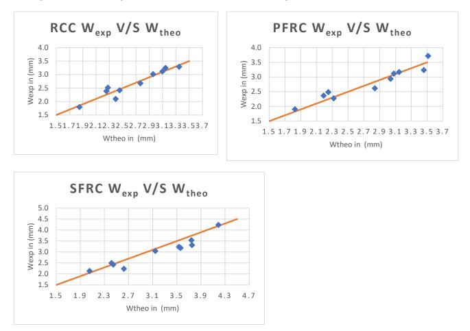
Comparison of experimental crack width Vs predicted values
