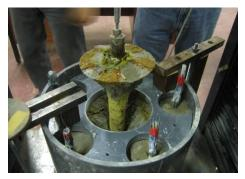
Fig. 2.33 Post electrokinetic treatment, (a) showing cementation spreading from the anode, (b) nail pullout test
