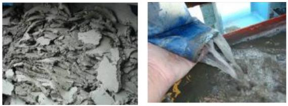
Fig. 2.27 Dewatered tailing (11V, 78% DS) and recovered water
