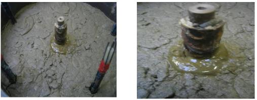
Fig. 2.32 Pullout of nail from tailings without electrokinetic treatment
