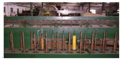
Fig. 5.5 Speed Frame Machine
