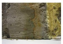
Fig. 2.35 Cementation of tailings radiating from the anode
