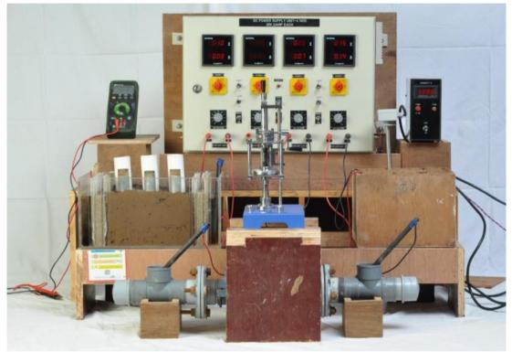
Fig. 4.5(b) Complete Setup of Electrokinetic Procedure
