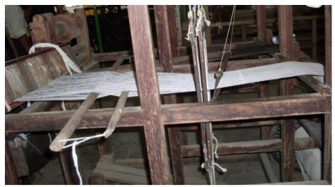
Fig. 5.14 Weaving Process on Handloom
