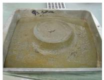
Fig. 2.31 Tailings at 17% moisture content liquefies when saturated (24% moisture content)
