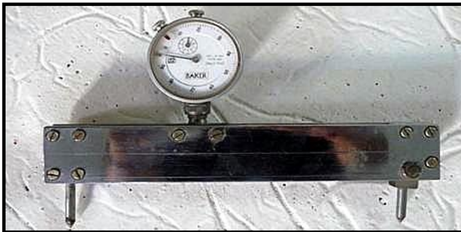
Fig. 1.4 Berry Type Mechanical Strain Gauge
