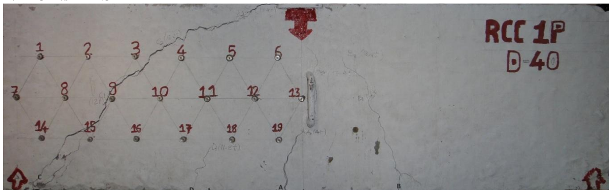
FIG. 6.82 D 40-S 0.0-RCC (WITHOUT STIRRUPS)-1P
