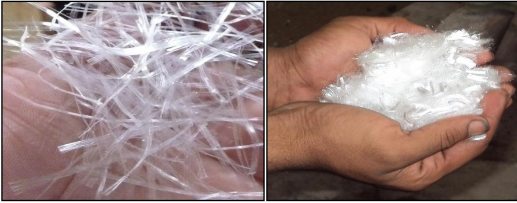
Fig. 3.1 Photographs Of Polypropylene Fibers (FT & MT respectively)
