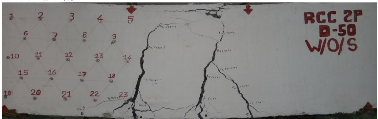
FIG. 6.87 D50-S 0.0-RCC (WITHOUT STIRRUPS)-2P
