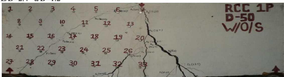
FIG. 6.83 D 50-S 0.0-RCC (WITHOUT STIRRUPS)-1P
