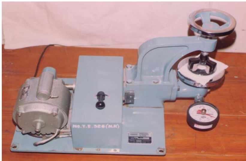
Photograph 3.3: Bursting strength test on Geotextile used in Sandwich
