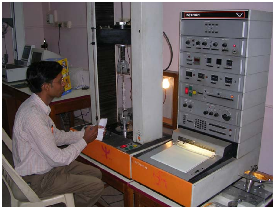
Photograph 3.1: Tensile test on geotextile used in fabricating Sandwich
