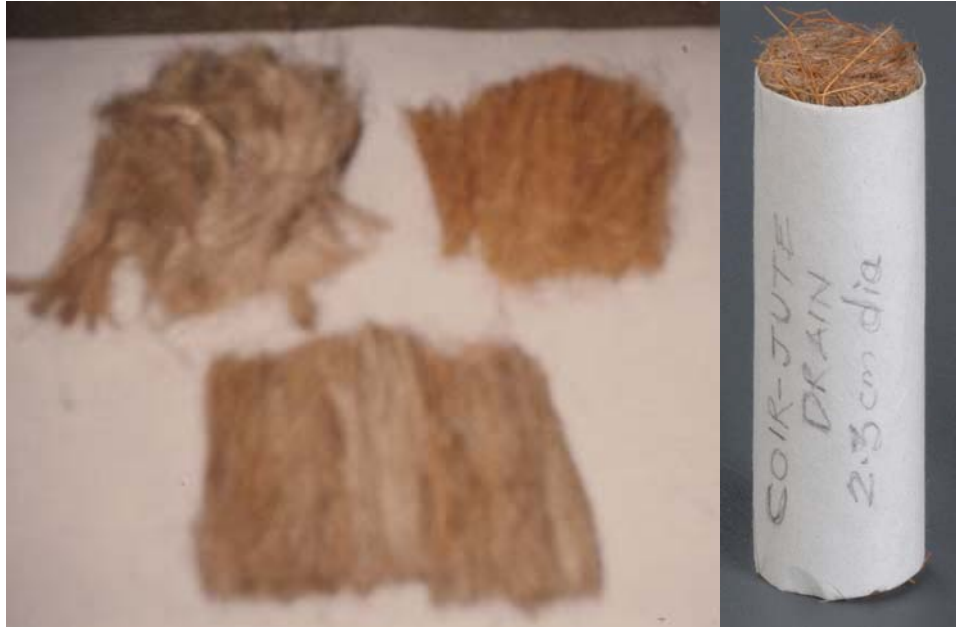
Photograph 3.5: Sample of Coir-Jute fibers and Coir-Jute drain ('n'11.04) encapsulated by filter paper
