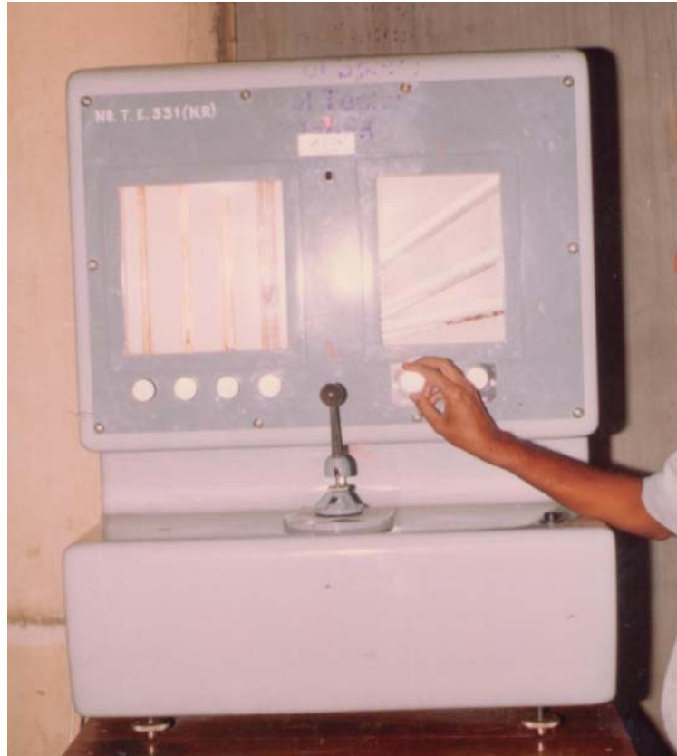
Photograph 3.2: Air permeability test on geotextile used in Sandwich
