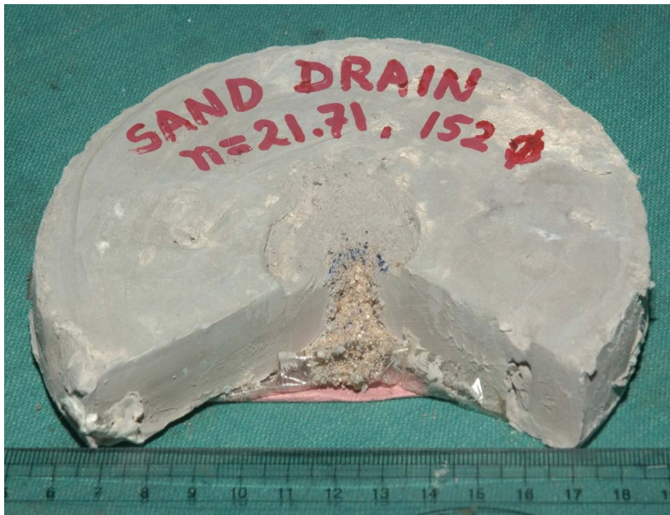
Photograph 6.22: Sectional view of consolidated clay sample (end of 320kPa pressure) with central vertical sand drain (SD) of n = 21.71
