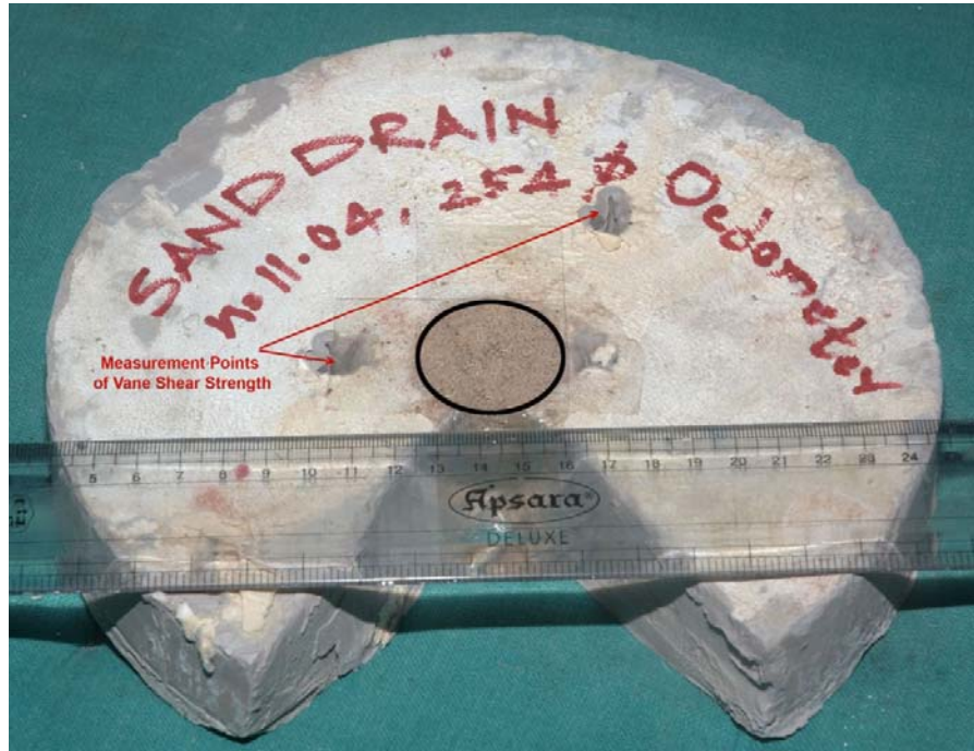
Photograph 6.9: Sectional view of consolidated clay sample (end of 320kPa pressure) with central vertical sand drain (SD) of n = 11.04
