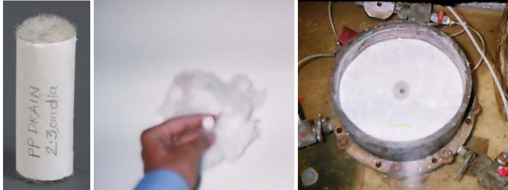
Photograph 5.13: Polypropylene fiber drain (PF) ready for installation and clay sample with central PF drain ready for testing
