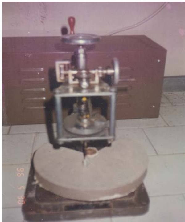
Photograph 5.7: Vane shear set-up with soil sample
