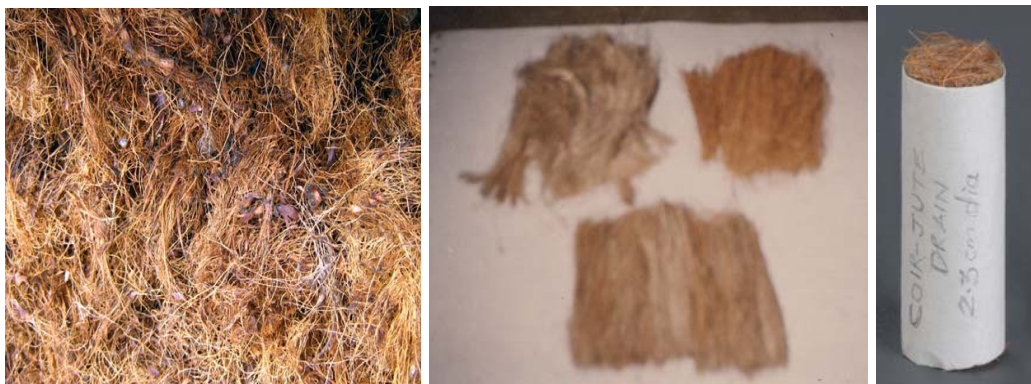
Photograph 5.12: Coir fibers, Bunch of coir and jute fibers of required length and coir-jute drain (CJ) of 'n'11.04
