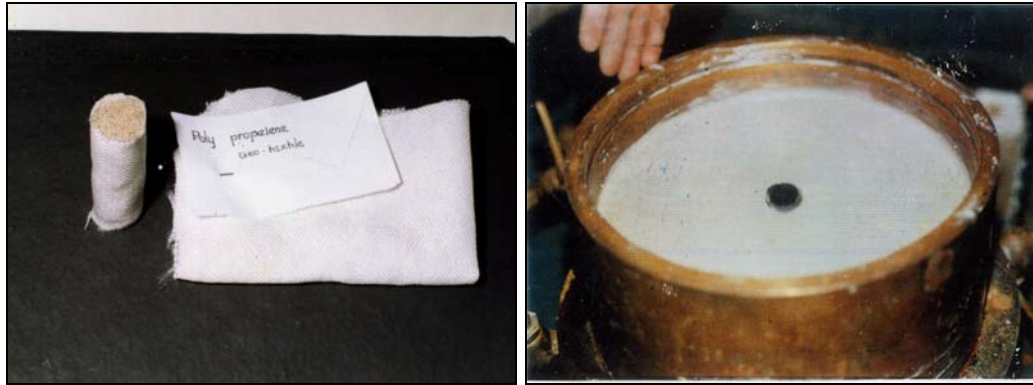
Photograph.5.11: Sandwich ('n'11.04) ready for installation and clay sample with central sandwich
