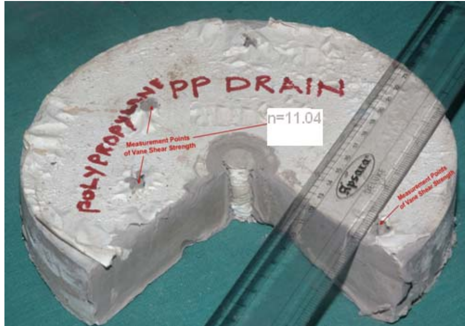
Photograph 6.12: Sectional view of consolidated clay sample (end of 320kPa pressure) with central vertical polypropylene fiber drain (PF) of n = 11.04
