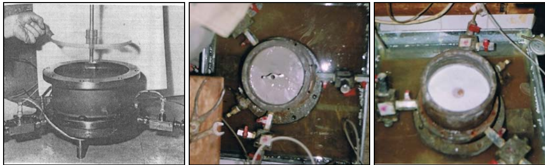
Photograph.5.9: Top platen installation, bore hole formation using circular mandrel and clay sample with central vertical sand drain ready for testing
