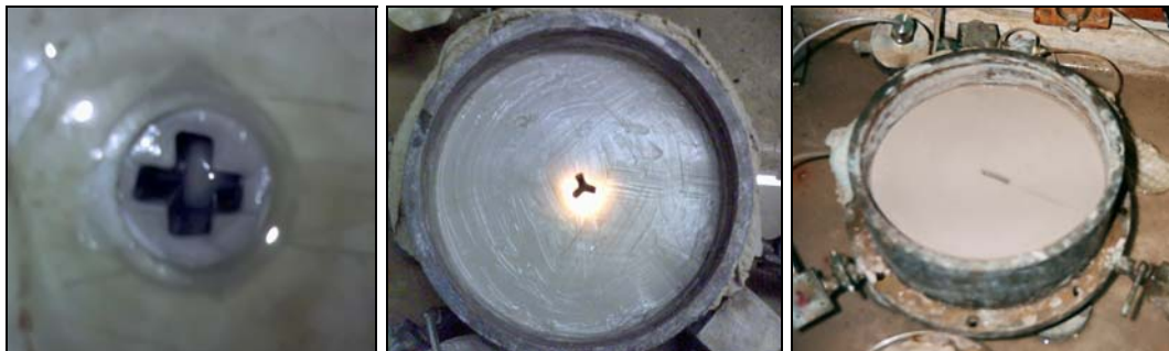
Photograph.5.10: Formation of plus shape , tripod shape and band shape bore hole using mandrel for geometrical shape sand drains
