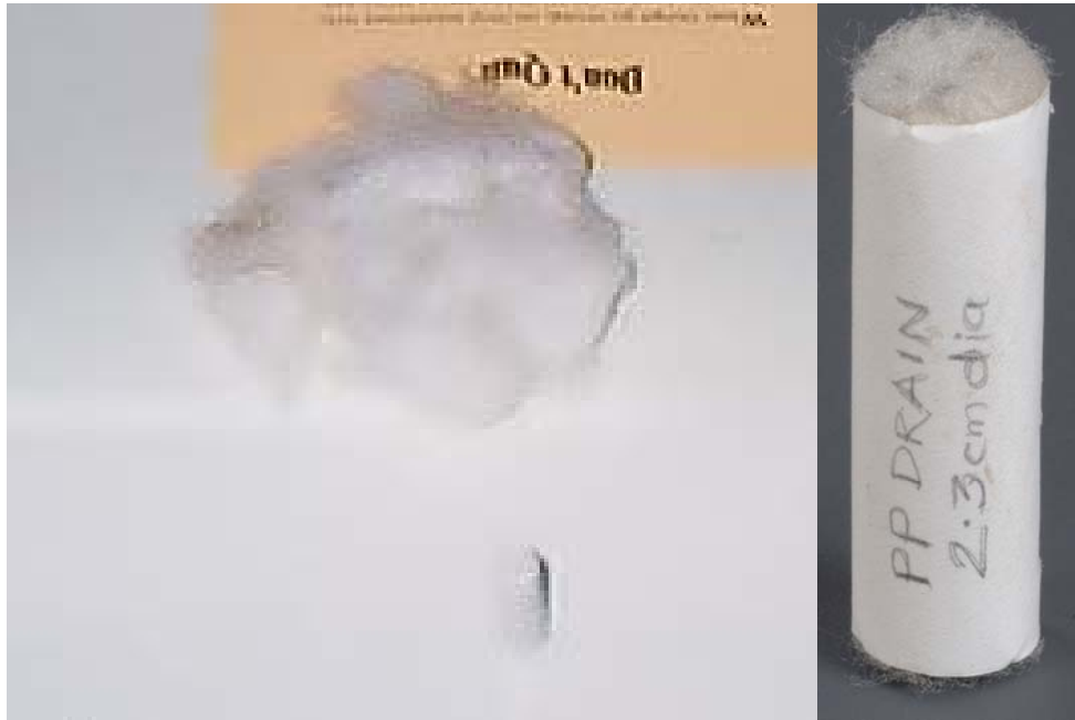
Photograph 3.6: Sample of white Polypropylene fibers and Polypropylene fiber drain ('n' 11.04) encapsulated by filter paper
