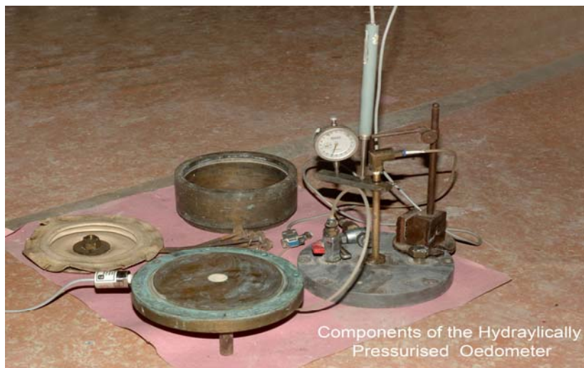
Photograph 5.3: Complete Oedometer assembly with its components
