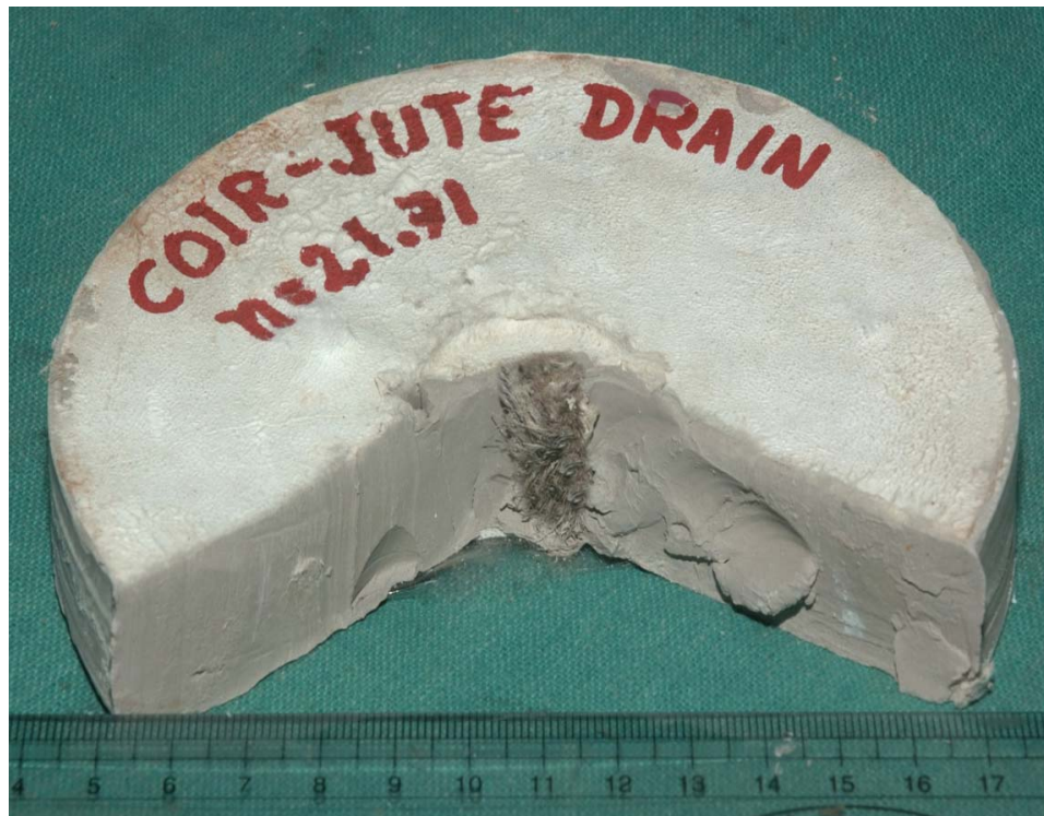
Photograph 6.24: Sectional view of consolidated clay sample (end of 320kPa pressure) with central vertical sand drain (CJ) of n = 21.71
