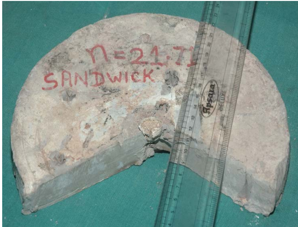
Photograph 6.23: Sectional view of consolidated clay sample (end of 320kPa pressure) with central vertical sand drain (SW) of n = 21.71
