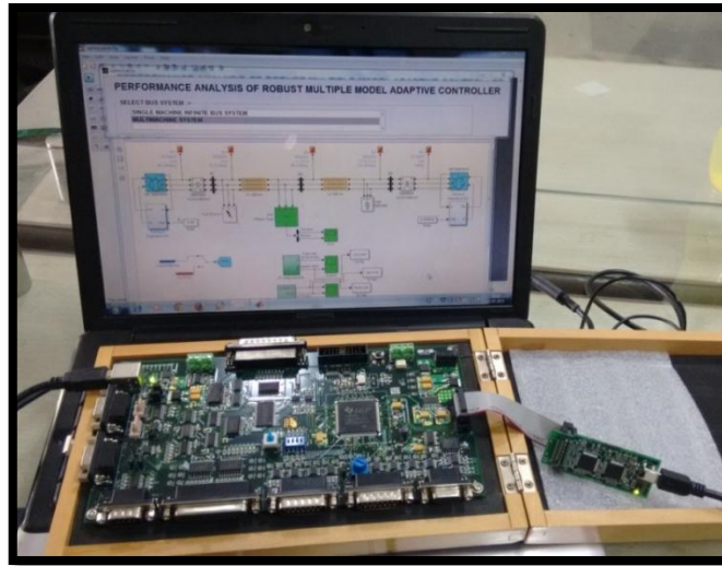
Fig. 5.11 Photograph of Hardware in loop configuration for Multimachine system
