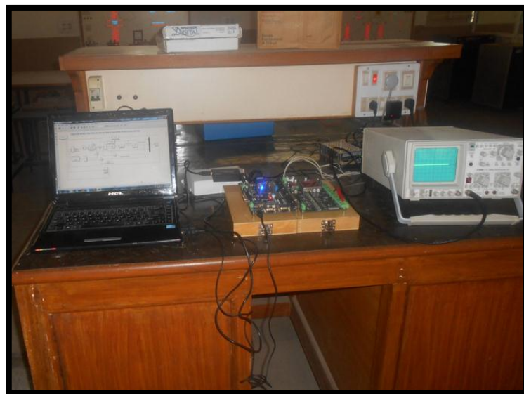
Fig. 5.6 Photograph of Hardware in loop configuration for SMIB system
