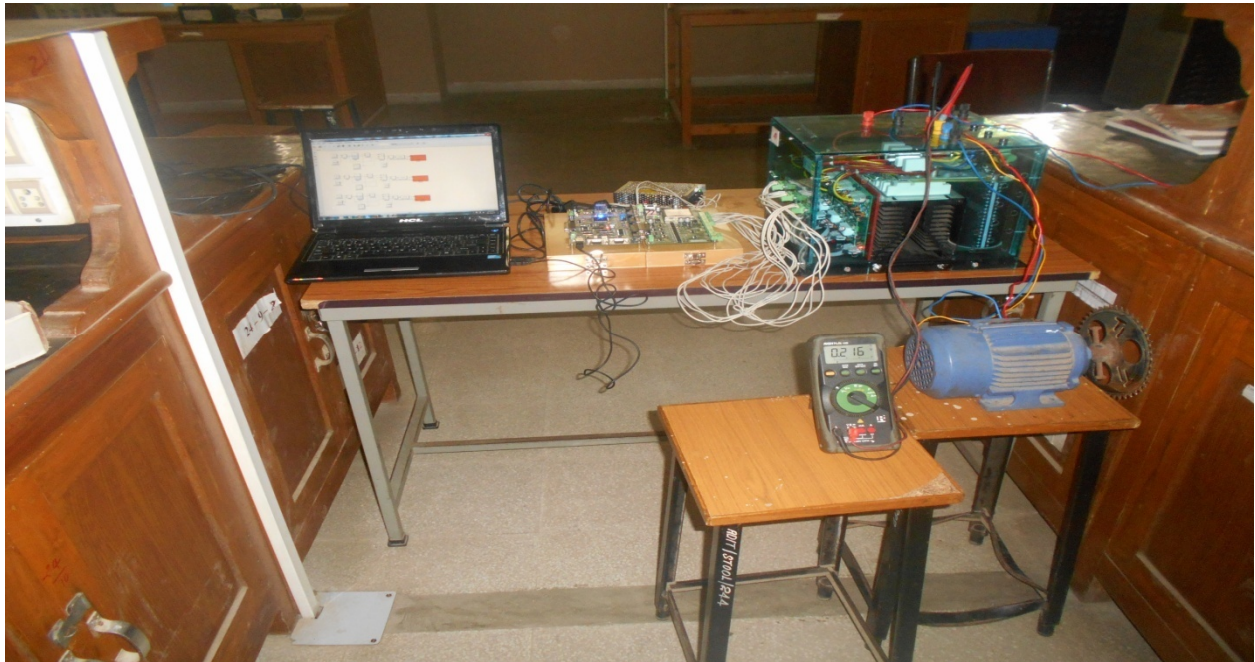
Figure 5. 15 Real time Experimental set up for SMC of Induction motor drive
