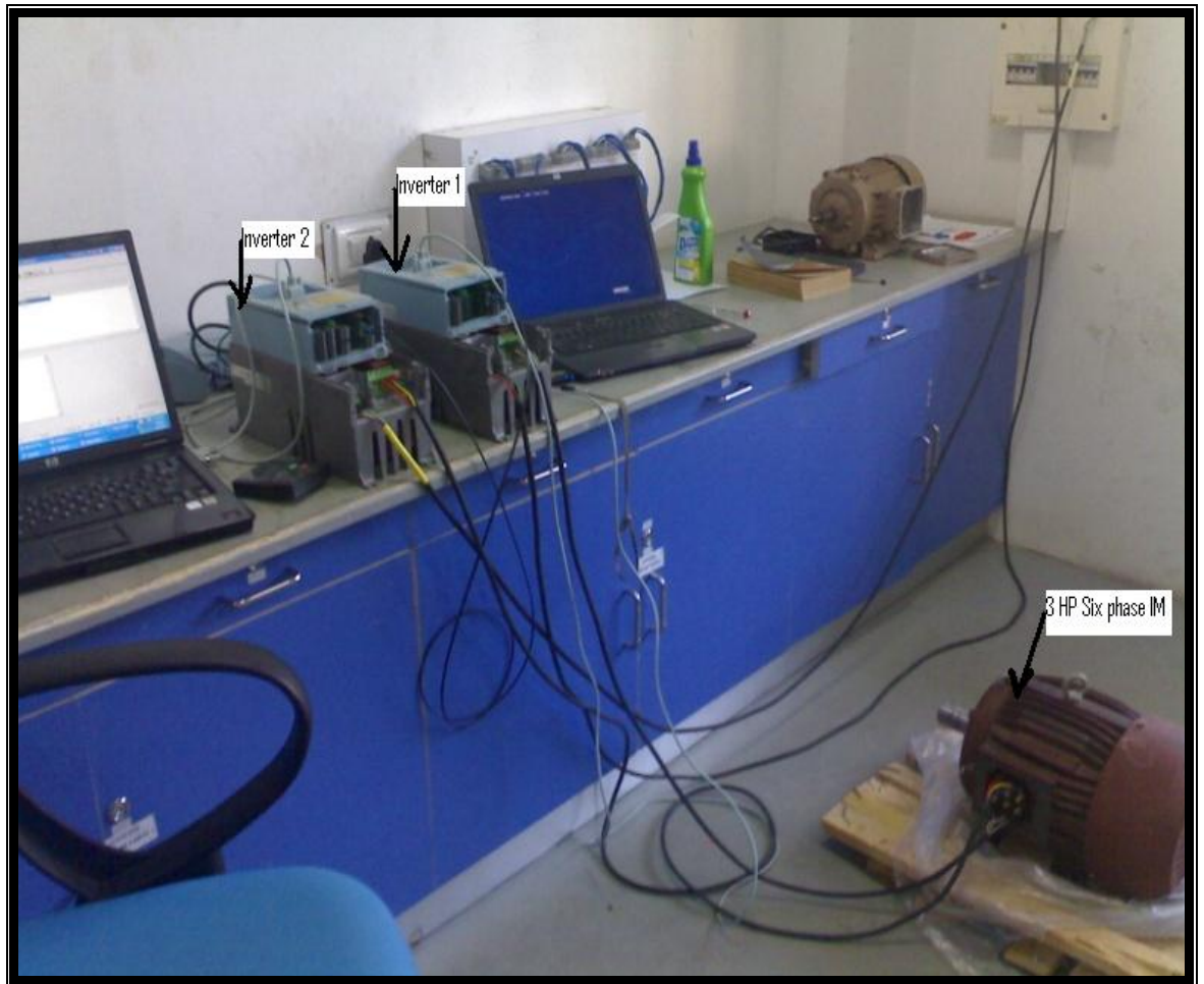
Photograph 6.1. Actual experimental set up for speed control of prototype six phase induction motor when fed from two, NXP drives at Chennai based Industry.
