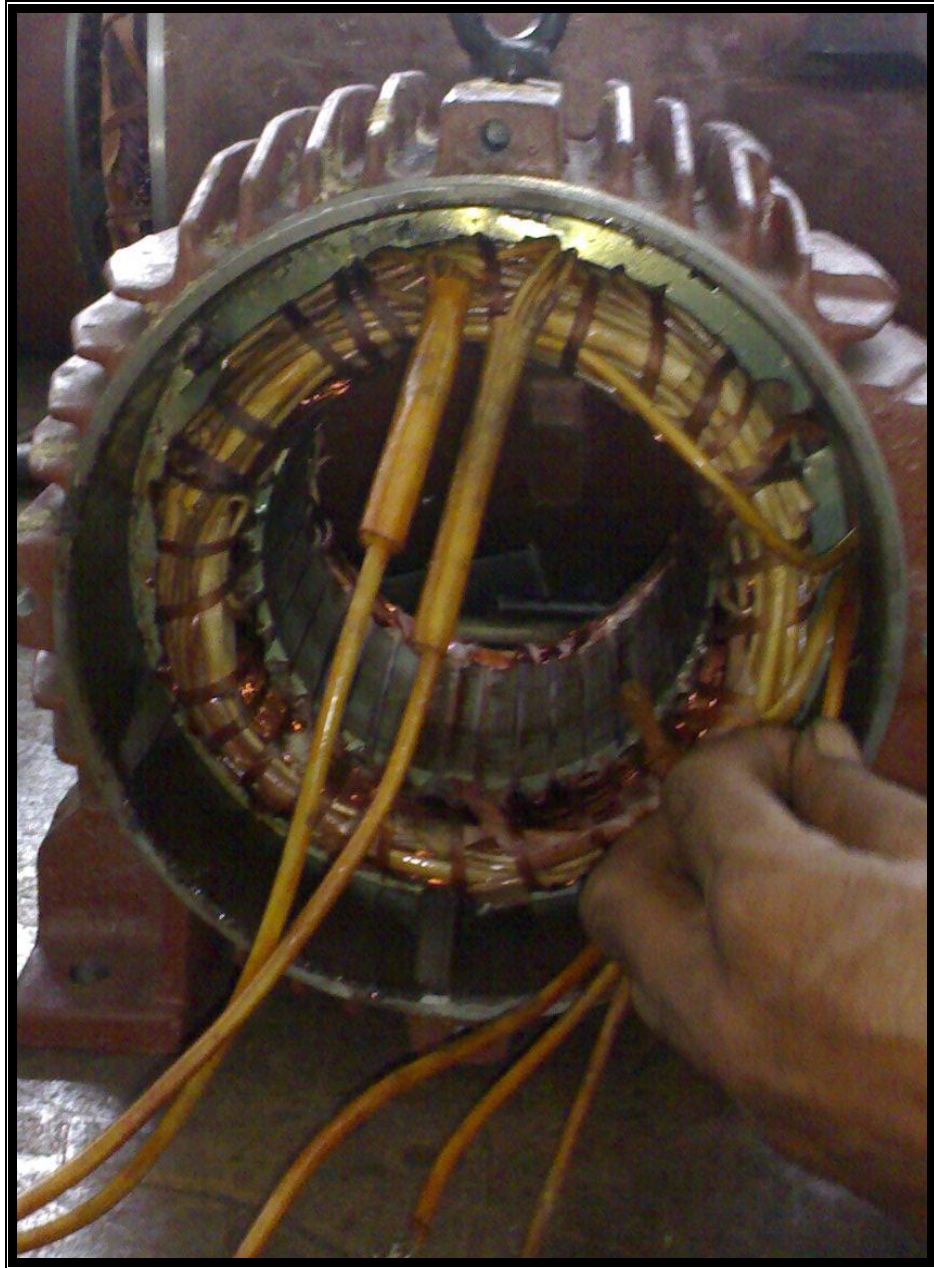
Photograph 3.2. Six phase stator after winding
