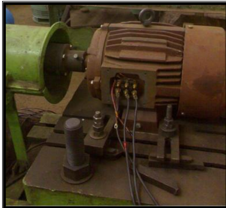
Photograph 3.8 Testing with shorted terminals
