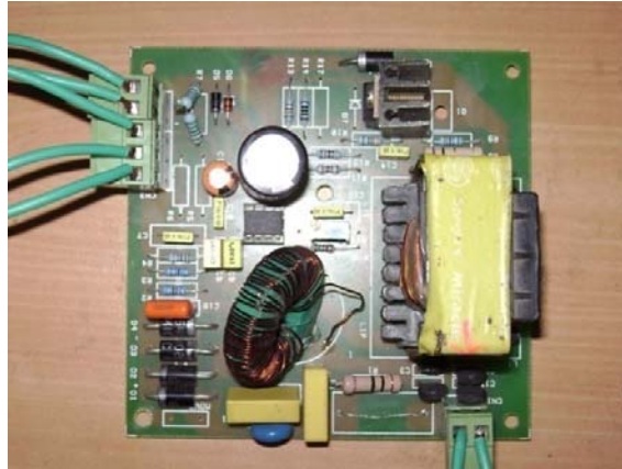
Figure 2.9.3-6: Rectifier with PFC assembled on PCB
