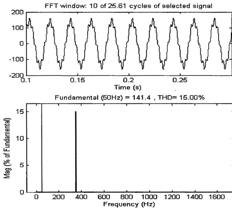
Fig 5.39 FFT analysis for source voltage
