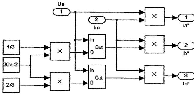
Fig 5.2 STATCOM Reference current generation
