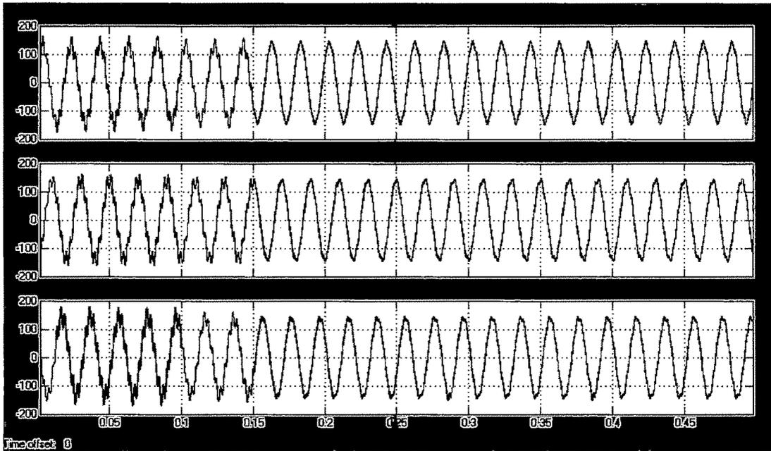
*Fig 5.33 Load voltage before and after compensation*
