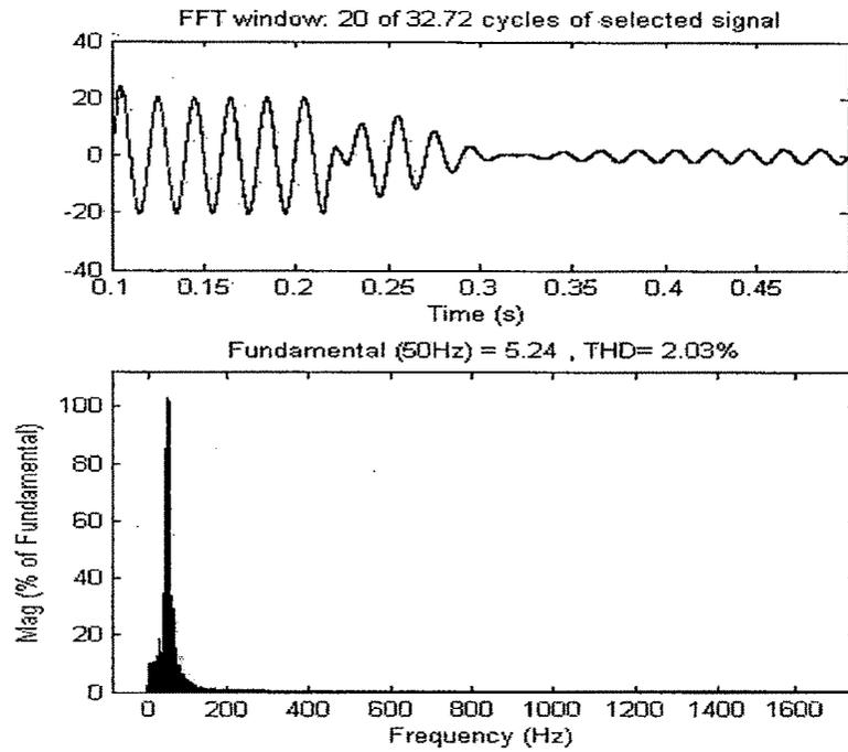
*Fig 5.20 FFT Analysis for source current*
