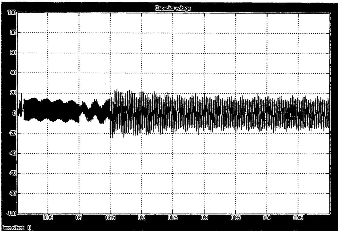
*Fig 5.34 Compensating voltage for phase 'A'*
