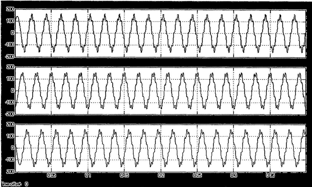
*Fig 5.24 Source voltage containing harmonics*
