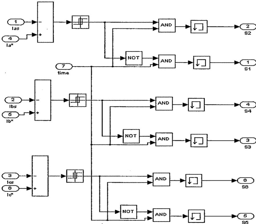
Fig 5.4 STATCOM Pulse generation diagram
