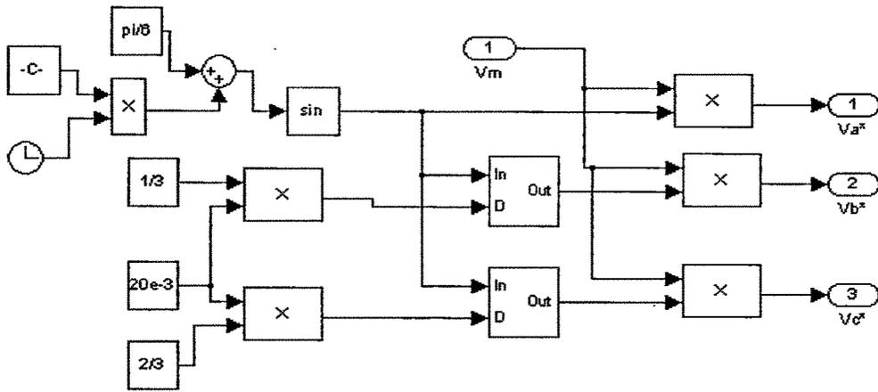
Fig 5.22 Reference voltage generation
