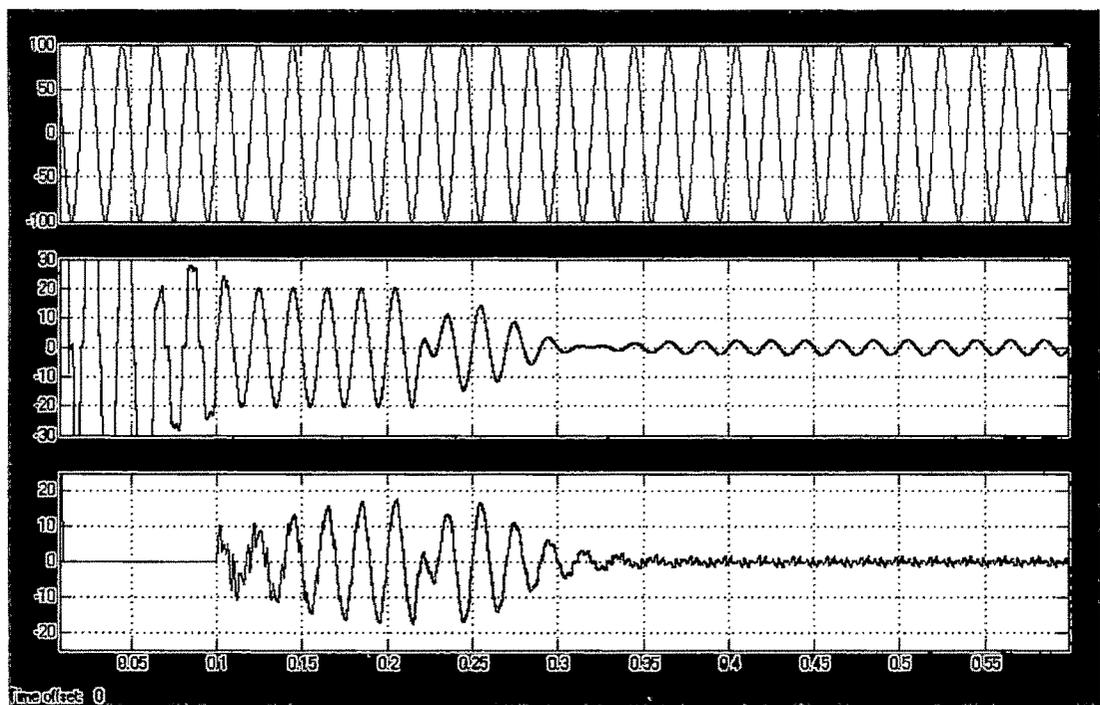
*Fig 5.17 Source voltage, source current and filter current*
