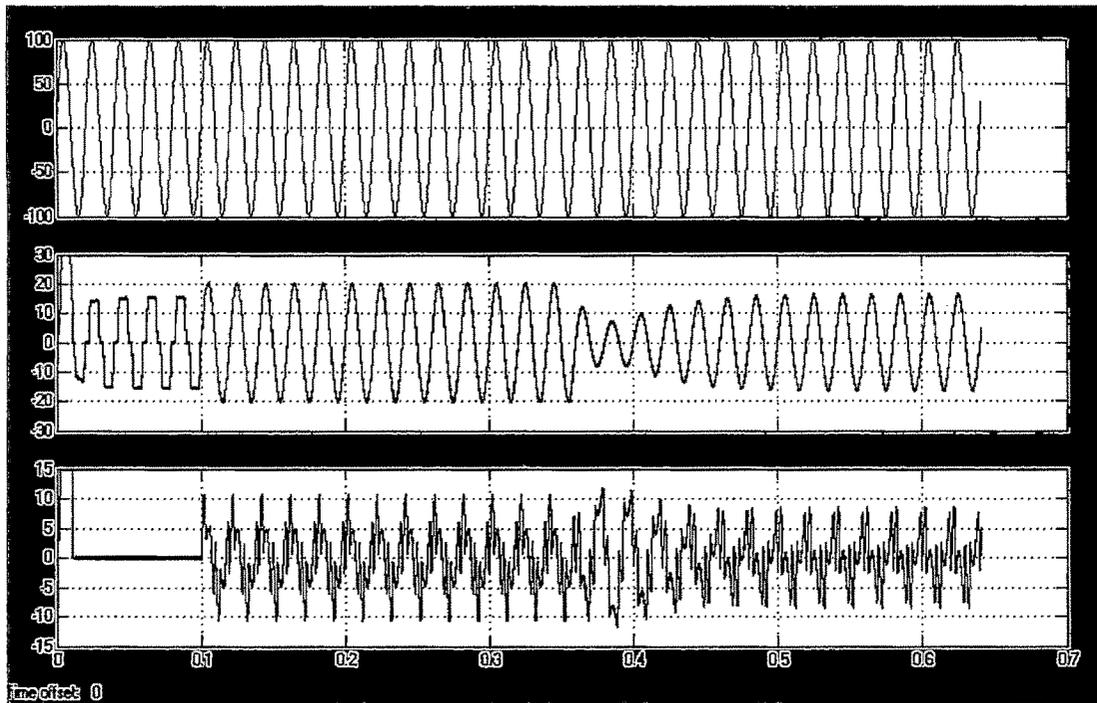
*Fig 5.9 Source voltage, source current and filter current for phase A*
