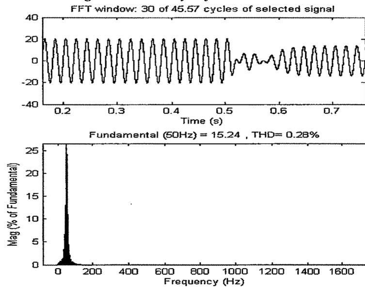
*Fig 5.51 FFT analysis for source current*
