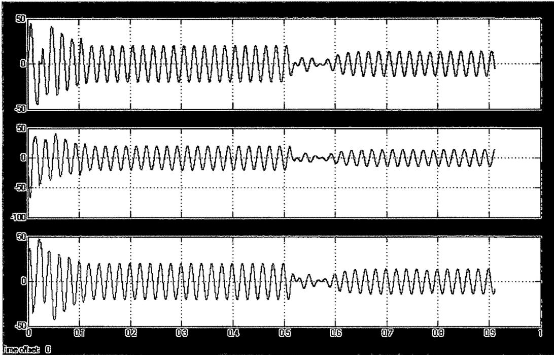
*Fig 5.46 Source current before and after compensation*
