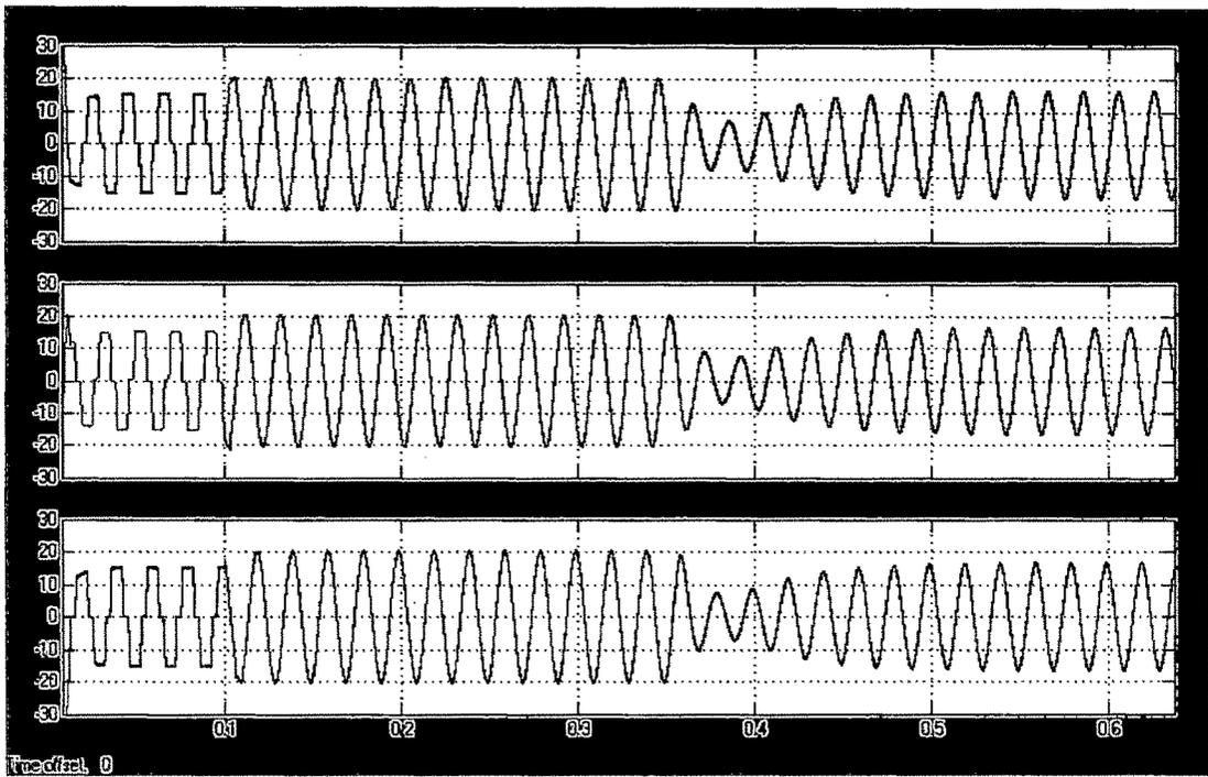
*Fig 5.8 Source current before and after compensation*
