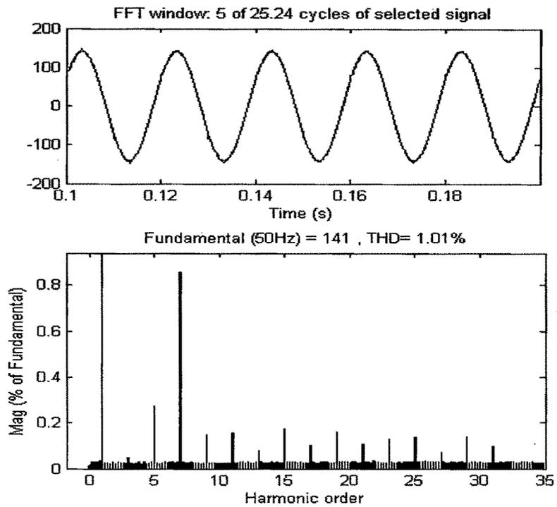
Fig 5.28 FFT Analysis for load voltage
