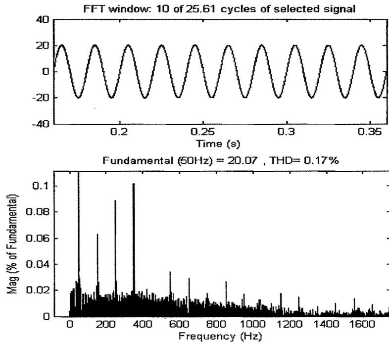
Fig 5.42 FFT analysis for source current
