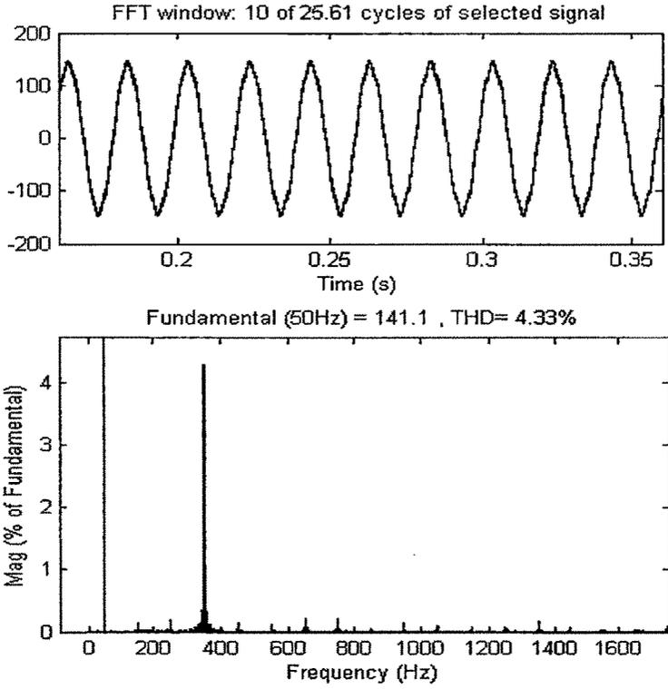
*Fig 5.40 FFT analysis for load voltage*
