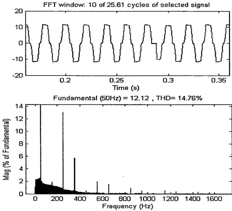
*Fig 5.41 FFT analysis for load current*
