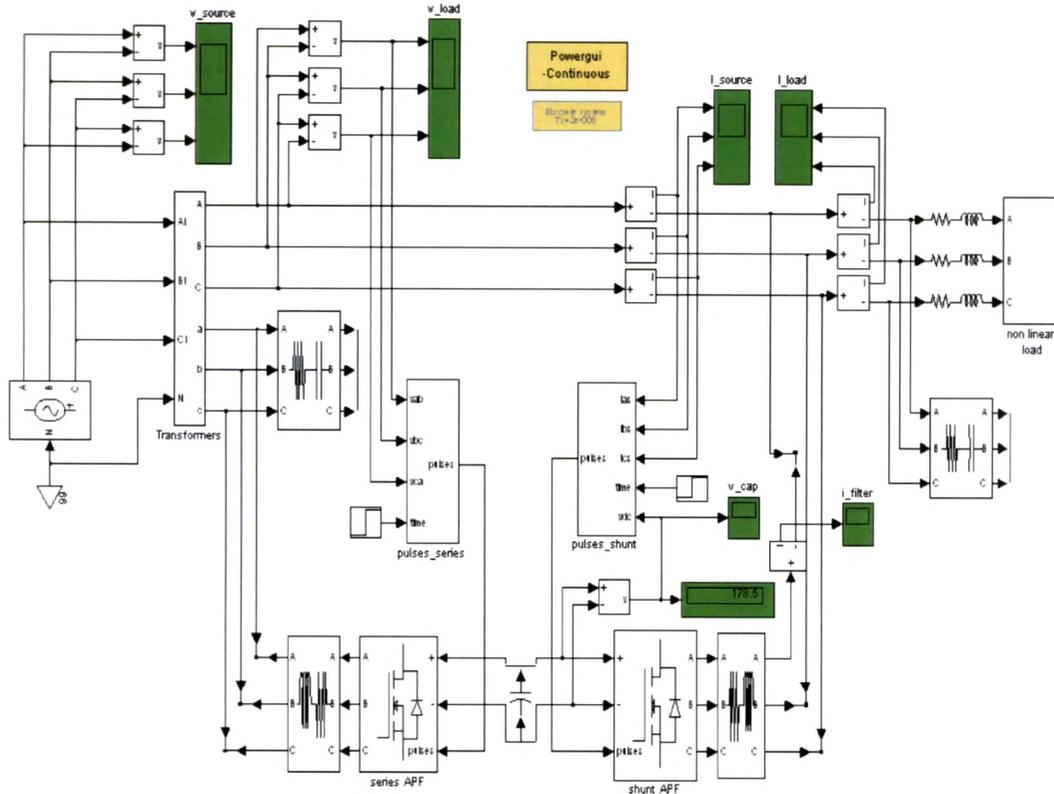
Fig 5.32 MATLAB model for Unified power quality conditioner (UPQC)
