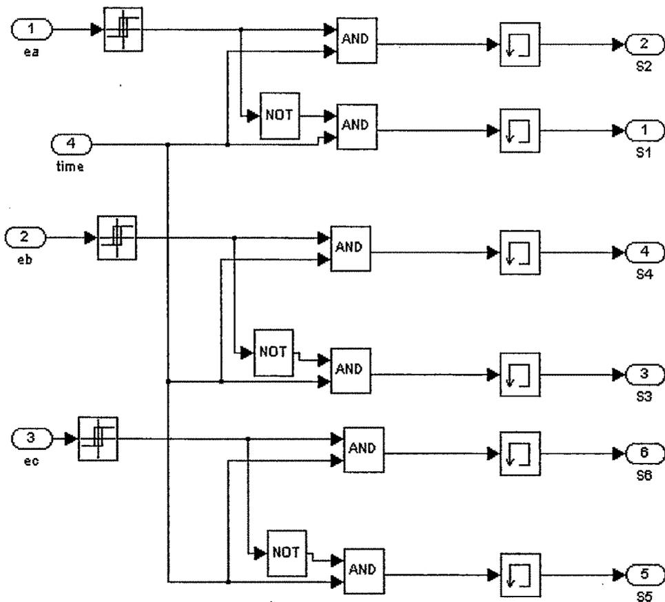
Fig 5.23 Pulse generation diagram
