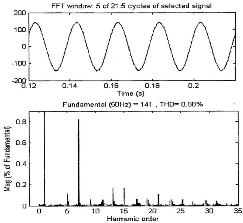
Fig 5.31 FFT analysis for load voltage
