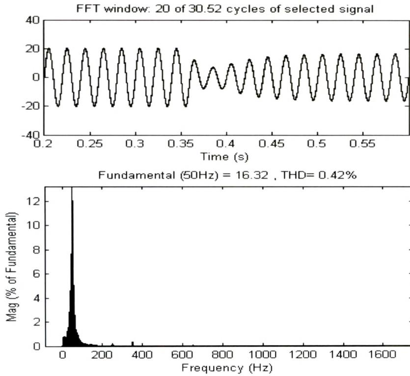
Fig 5.12 FFT Analysis for source current
