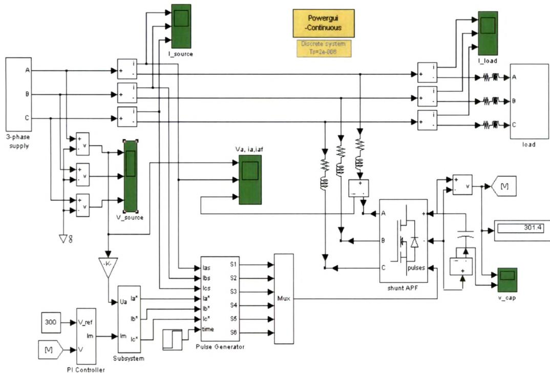
Fig 5.1 MATLAB model for *Shunt* active power filter
