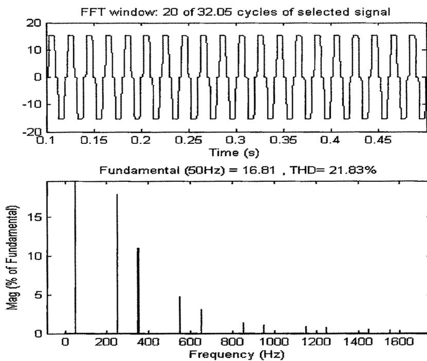
Fig 5.11 FFT Analysis for load current
