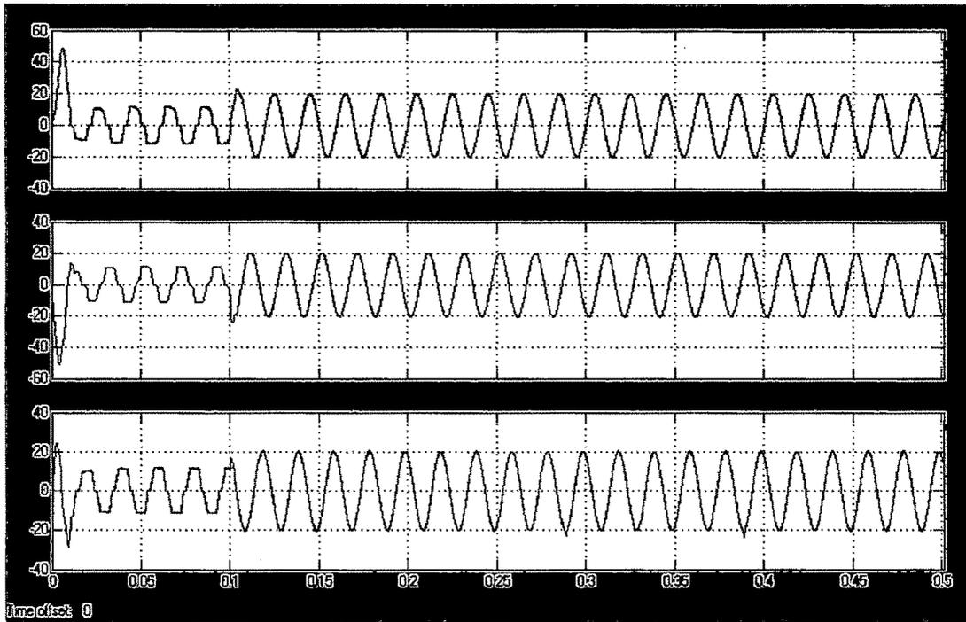
*Fig 5.36 Source current before and after compensation*
