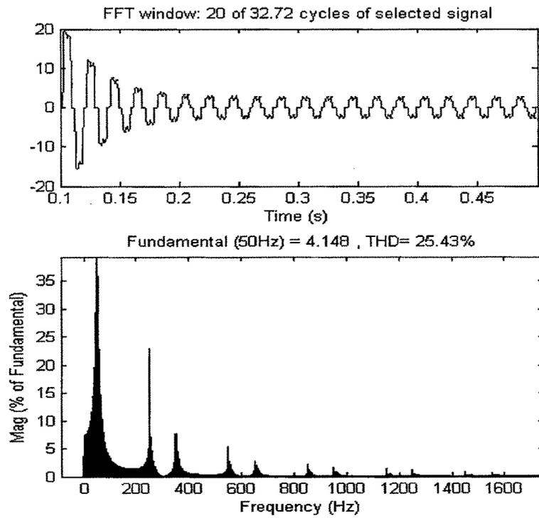
Fig 5.19 FFT Analysis for load current
