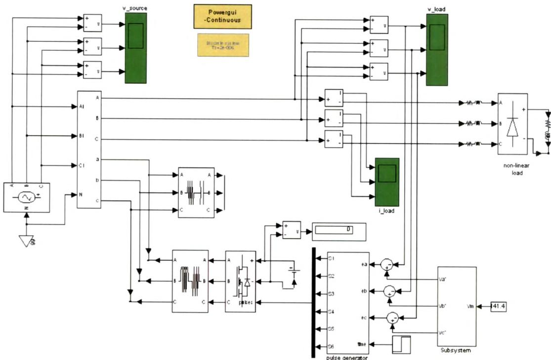
Fig 5.21 MATLAB model for *Series* active power filter
