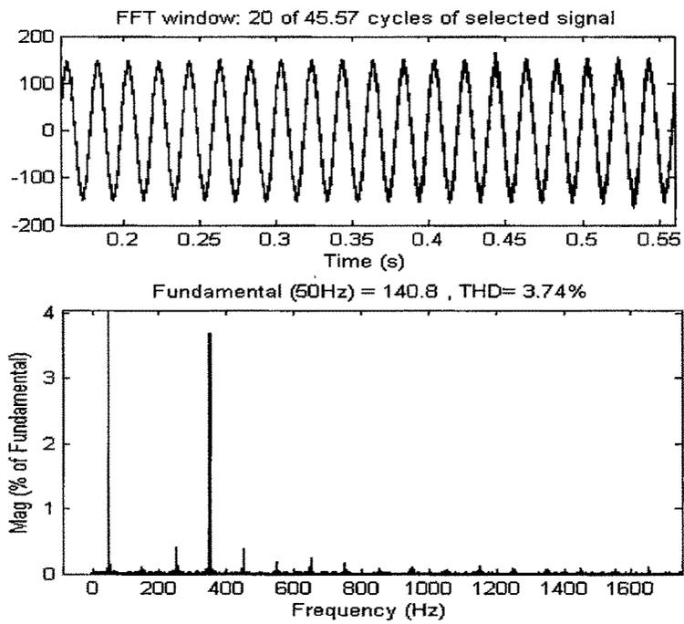
Fig 5.49 FFT analysis for load voltage
