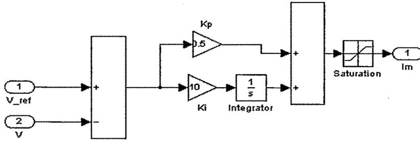
Fig 5.3 Calculation of maximum value of reference current using PI controller
