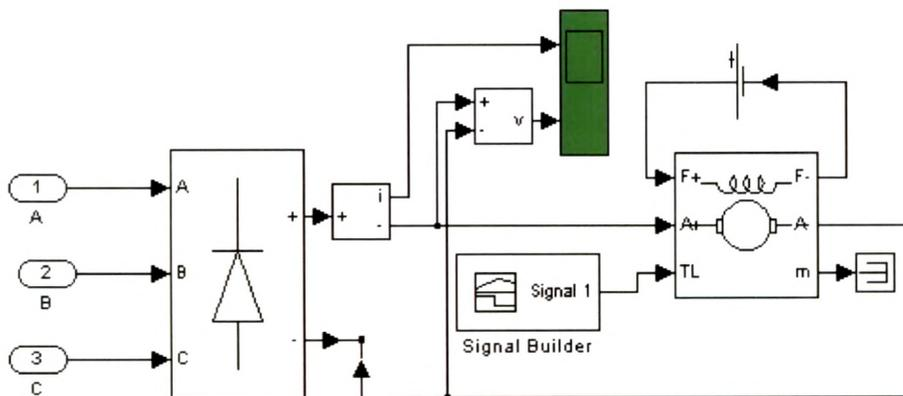
Fig 5.13 DC machine with variable load torque
