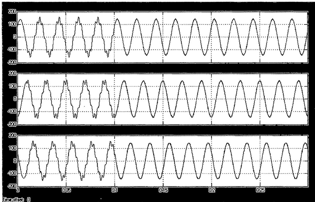
*Fig 5.25 Load voltage before and after compensation*
