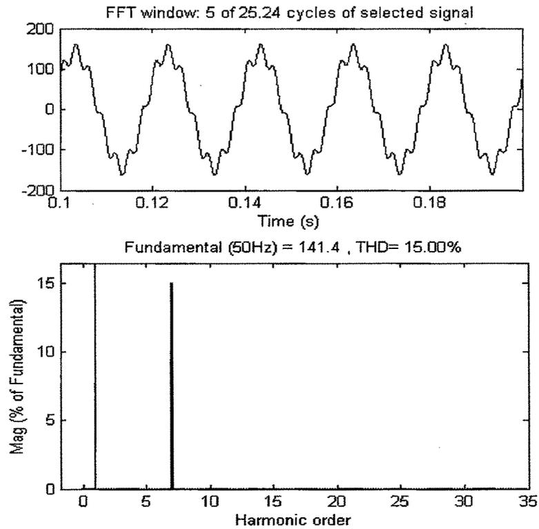
Fig 5.27 FFT Analysis for source voltage
