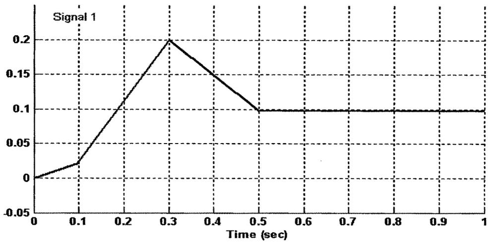
Fig 5.14 Waveform of the torque applied to dc machine
