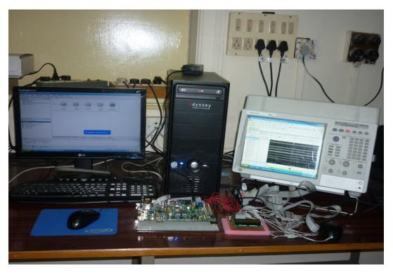
**B-III: System Setup for FPGA Implementation of ANN**
