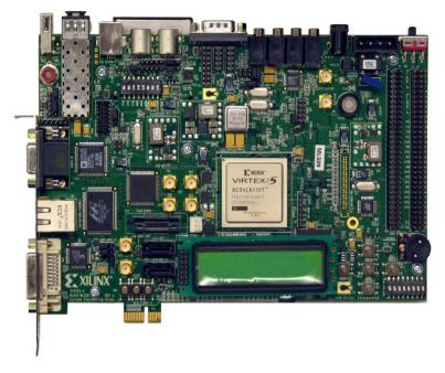
Figure A.13 (a): Snap Shot of XCV5LX110T FPGA Board
