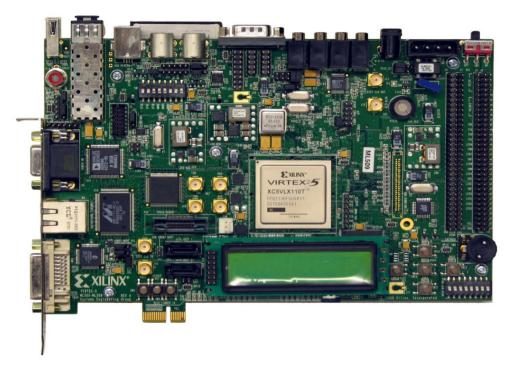
**B-II: XCV5LX110T FPGA Evaluation Board: Front View**
