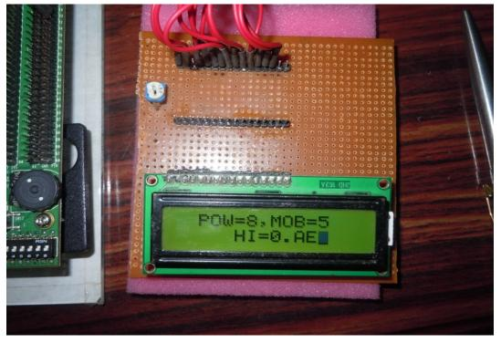
**B-VII: Output displayed on LCD for Different Inputs of Purelin ANN**
