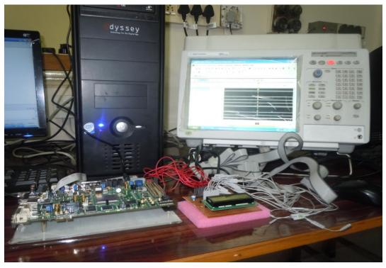
**B-VI: Output Observed on GPIO for Different Inputs using Logic Analyzer**
