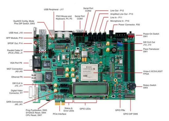
Figure A.13 (b): Snap Shot of XCV5LX110T FPGA Board with peripherals
