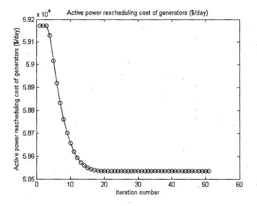
Figure 6.5: Convergence characteristic of PSO for active power rescheduling cost of 75-bus system(Output of all generators are rescheduled)
