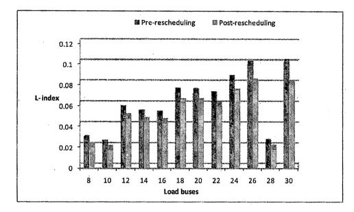
Figure 6.1: L-index values of some load buses before and after rescheduling for IEEE 30 bus system
