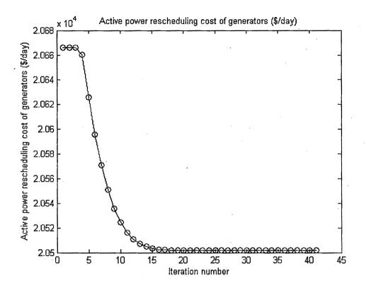
Figure 6.6: Convergence characteristic of PSO for active power rescheduling cost of 75-bus system(Output of only selected generators are rescheduled)
