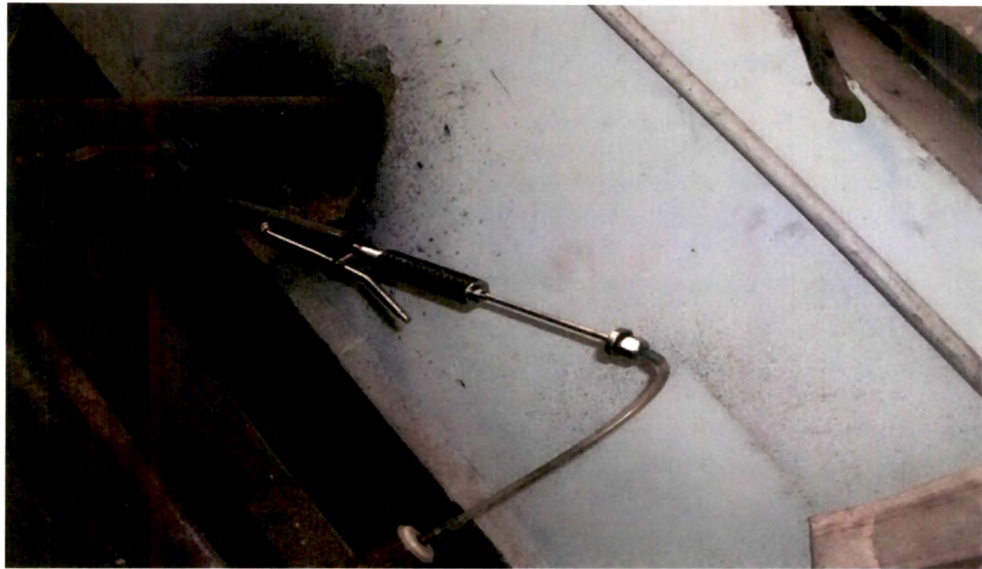
Plate 3.19 Measurement of Exhaust Gas Constituents
