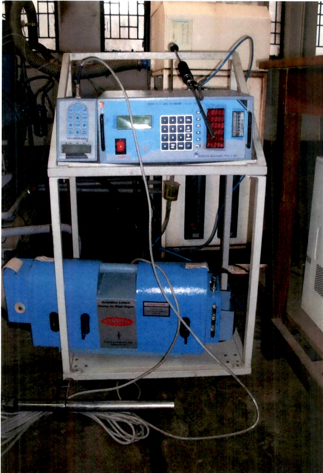
Plate 3.17 Assembly of Emission Measurement Systems
