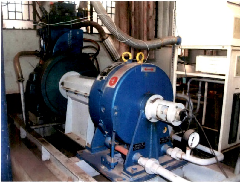
Plate 3.8 Assembly of Eddy Current Dynamometer and Engine
