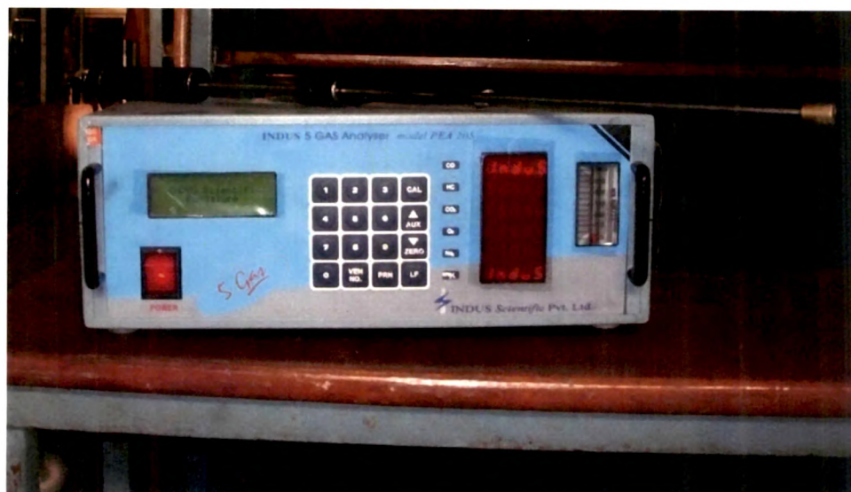
Plate 3.18 Exhaust Gas Analyzer
