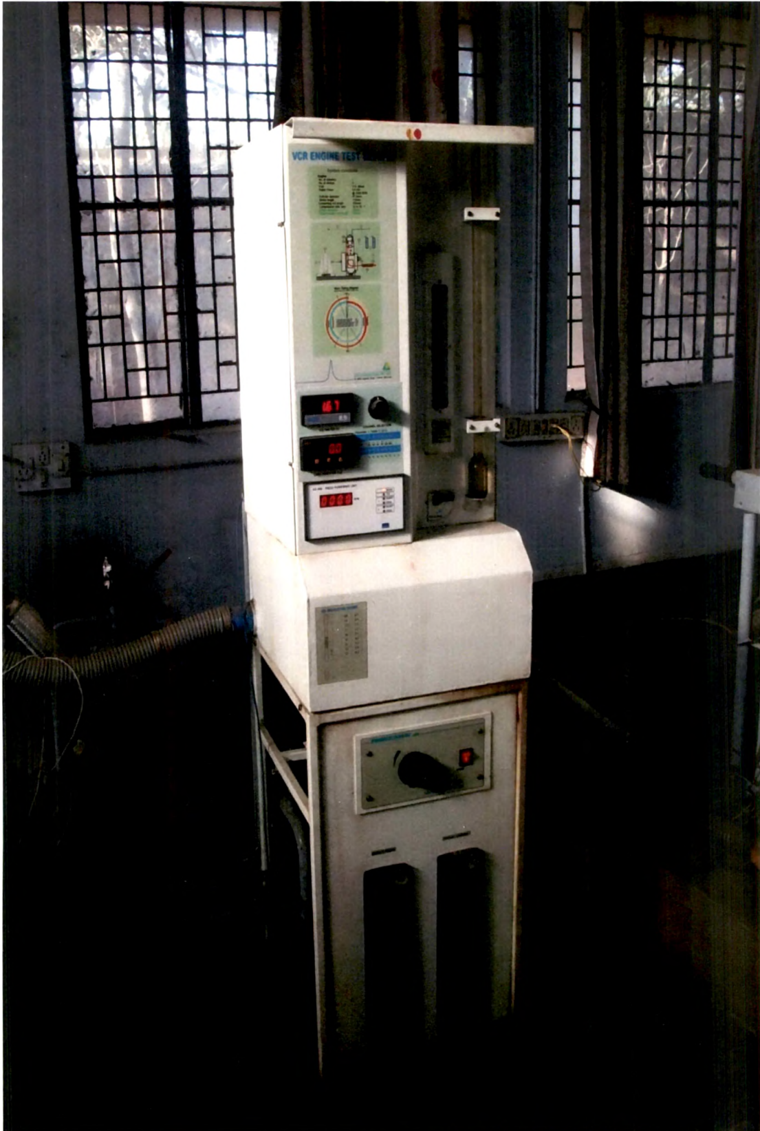
Plate 3.12 Engine Panel Box
