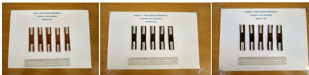
Figure 4.11 Post cured Specimens of jute, basalt and Carbon fibers with vinyl ester as per ASTM 790 for flexural test
