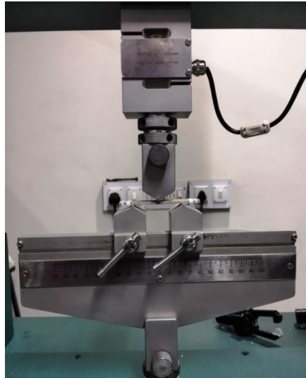
Figure 4.6 Flexural Testing in Universal Testing Machine (Model: TINIUS OLSEN/LSeries H50KL)
