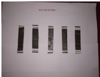
Figure 4.13 (a) Specimens with SiC Filler (b) Specimen with Cu Filler (c) Specimen with Al Filler as per ASTM 790 for flexural tests
