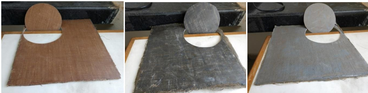
Figure 4.22 Specimen for testing thermal conductivity of Jute-Polyester composite as per ASTM C1530 (a) with Cu Filler (b) with SiC Filler (c) with Al Filler
