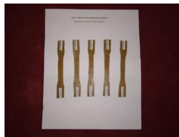
Figure 4.9 Specimens of in-process curing for tensile test as per ASTM 638 standards
