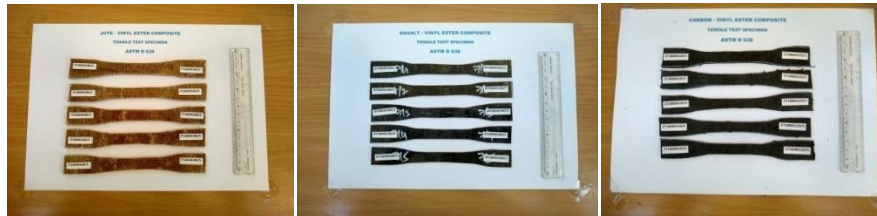
Figure 4.8 Post cured Specimens of jute, basalt, and Carbon fibers with vinyl ester as per ASTM 638 for tensile tests
