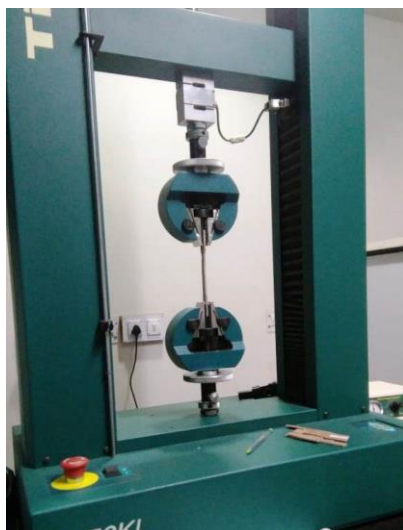
Figure 4.5 Tensile Testing in Universal Testing Machine (UTM) (Model: TINIUS OLSEN/LSeries H50KL)
