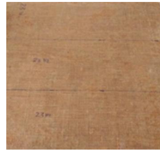
Figure 4.7 (c) Plate of Jute-Vinyl Ester Post Cured
