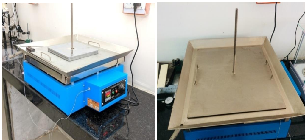
Figure 4.2 Developed Punch and Mould Assembly with Hot Plate for In-Process Curing
