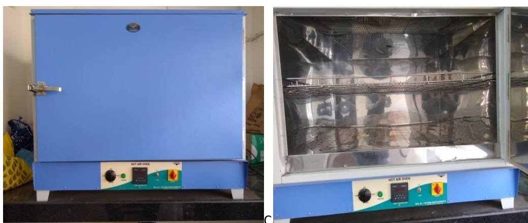
Figure 4.1 Developed Hot Air Oven for Post-Process Curing
