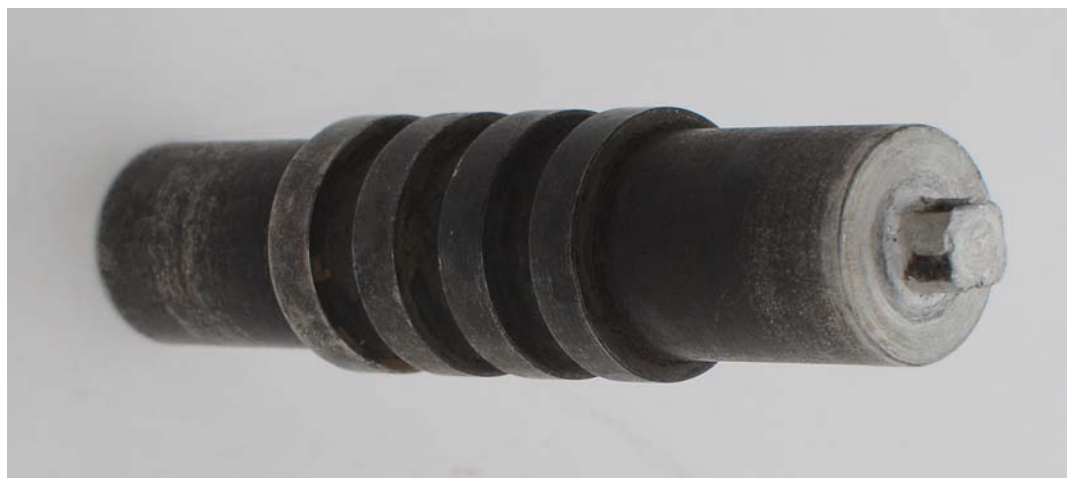
Figure 3.20: Tool geometry used for the friction stir welding of AA 6101 T6 alloy - Square pin profile with flat shoulder (C2)
