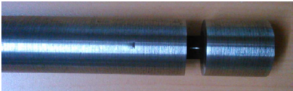
Figure 3.24: Fixed gap bobbin tool with square pin, concave-convex shoulder BT1
