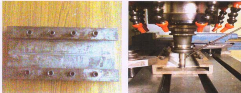
Fig.5. Fixture with horizontal movement restricted in X-direction and vertical clamping at edge [6]
