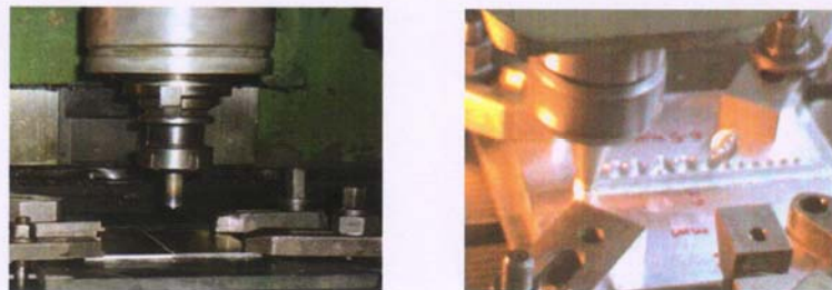
Fig.6. Clamping of plates using workshop clamps [7, 8]
