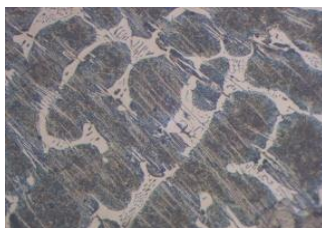
Fig. 5.12: Microstructure of product by addition of Vizag Sludge composite pellet to the melt at 17.66 pct (100X)
