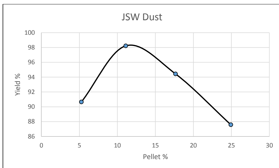
Fig. 5.3: Iron yield variation with addition of JSW Dust composite pellet
