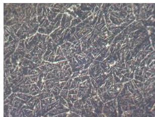
Fig. 5.11: Microstructure of product by addition of JSW Sludge composite pellet to the melt at 11.33 pct (100X)
