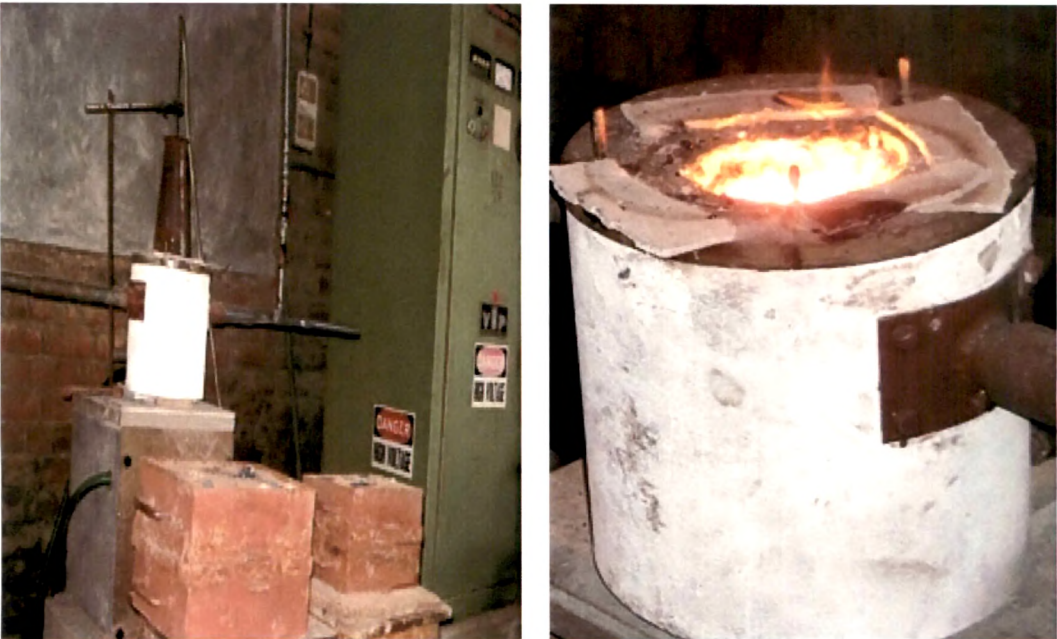
Photo 4.1: Smelting reduction set-up (induction furnace with power control panel).
