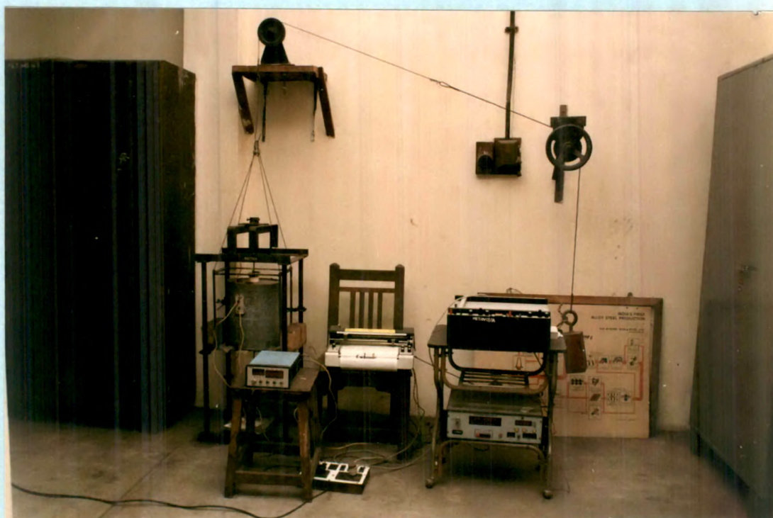
Fig. 3.4 Set-up for measurement of thermal diffusivity
