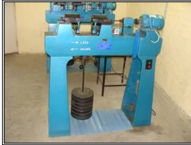
Figure: 2 Pictorial view of rotating bending fatigue machine
