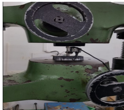
Fig. 4.8 Specimen under Tensile load Press capacity 60 Ton Capacity
