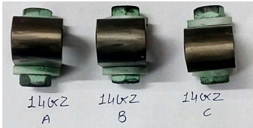
Fig. 4.29 No Crack appears in 10 Ni 22 Cr Weld Sample
