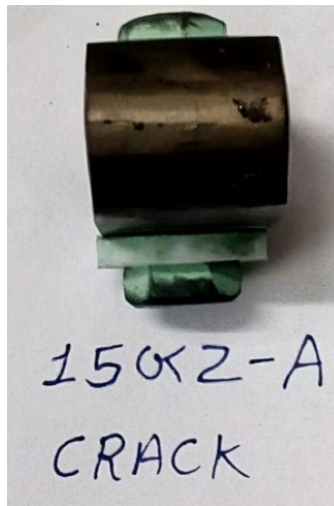
Fig. 4.31 Crack appears in 11 Ni 22 Cr Weld Sample
