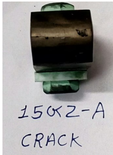
Fig. 4.32 Crack appears in 11 Ni 22 Cr Weld Sample
