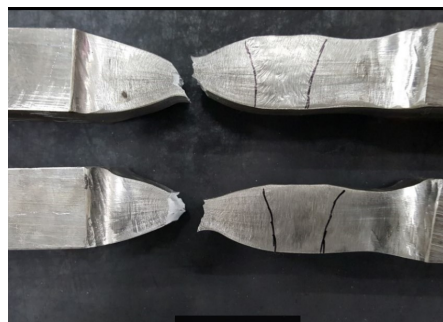
Fig. 4.10 Fractured specimen shows fracture from the P.M.
