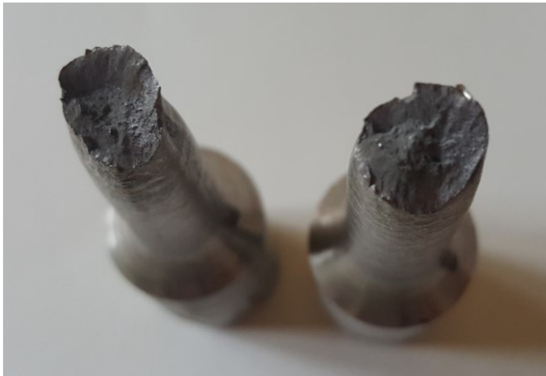
Fig.4.2 Ductile fracture within Gauge length for all weld test Coupons
