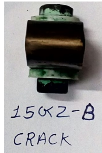
Fig. 4.33 Crack appears in 11 Ni 22 Cr Weld Sample
