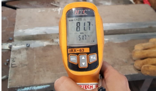
Figure 19 Use of digital thermometer to control less than 150 °C inter pass temperature.
