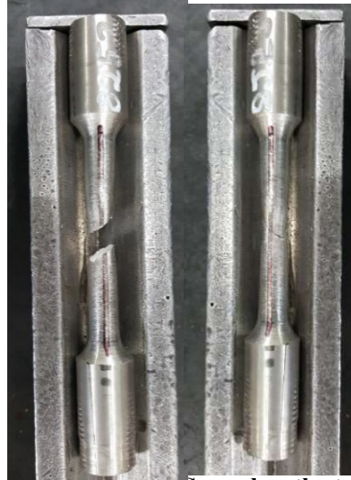
Fracture within Gauge length at 91740 N
