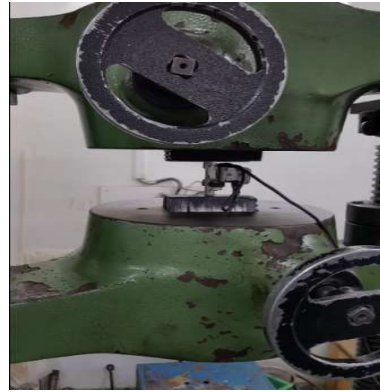
Figure 24 Specimen under Tensile load Press capacity 60 Ton Capacity
