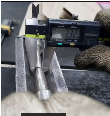
Figure 29 Final Diameter 7.32 mm measurement.
