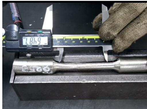
Fracture within Gauge length at 91740 N
