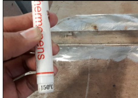
Figure 20 Use of templistic to control less than 150 °C inter pass temperature.
