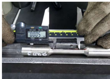
Figure 27 Initial gauge length measurement ~ 50 mm
