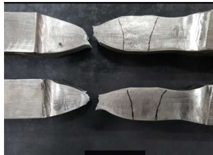
Figure 25 Fractured specimen shows fracture from the P.M.
