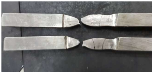
Figure 23 Transverse Tensile Specimen After fracture
