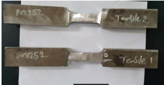
Figure 22 Transverse Tensile Specimen before fracture
