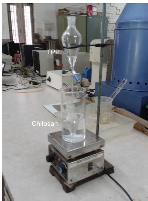
Figure 3.7 Experimental set up for the preparation of nano chitosan by ionic gelation method
