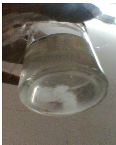
Figure 3.15 Stability study: white globular residue formed by microbial attack on CHTN
