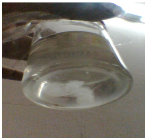
Figure-8 Stability study: white globular residue formed by microbial attack on CHT1N
