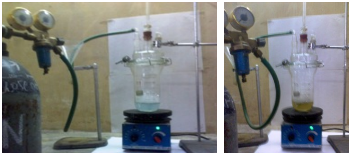
Figure 2.1 Experimental setup; reaction chamber with N 2 gas supply
