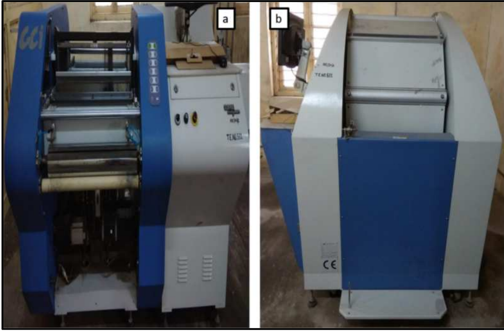
Figure 3.4: (a) CCI Rigid rapier loom and (b) CCI single end warping machine
