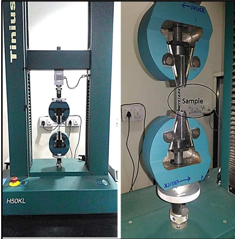
Figure 3.26a: Universal Testing Machine by TINIUS OLSEN/L-Series H50KL (Left); Sample fixture (Right)
