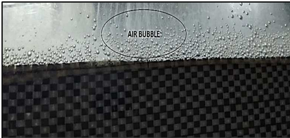
Figure 3.19: Image showing air bubble squeezed out of composite
