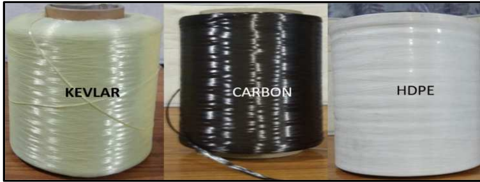
Figure 3.1: Kevlar, Carbon, and HDPE yarn package (from L to R)
