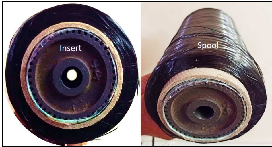
Figure 3.5: Arrangement on package for side withdrawal on CCI single end warping machine
