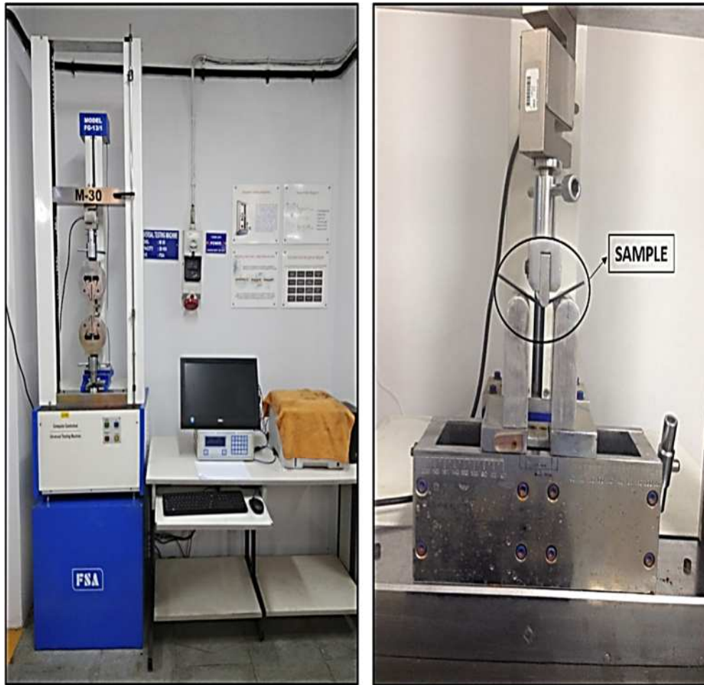
Figure 3.30: FSA Model M-30 (FG-13/1) UTM (Left); Sample Fixture (Right).
