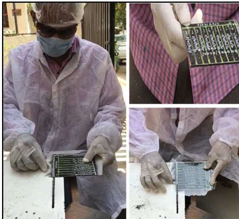
Figure 3.22: Arrangement for cutting of composite samples
