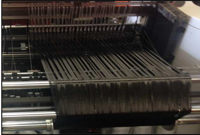
Figure 3.6: Path of the warp at the back of the loom
