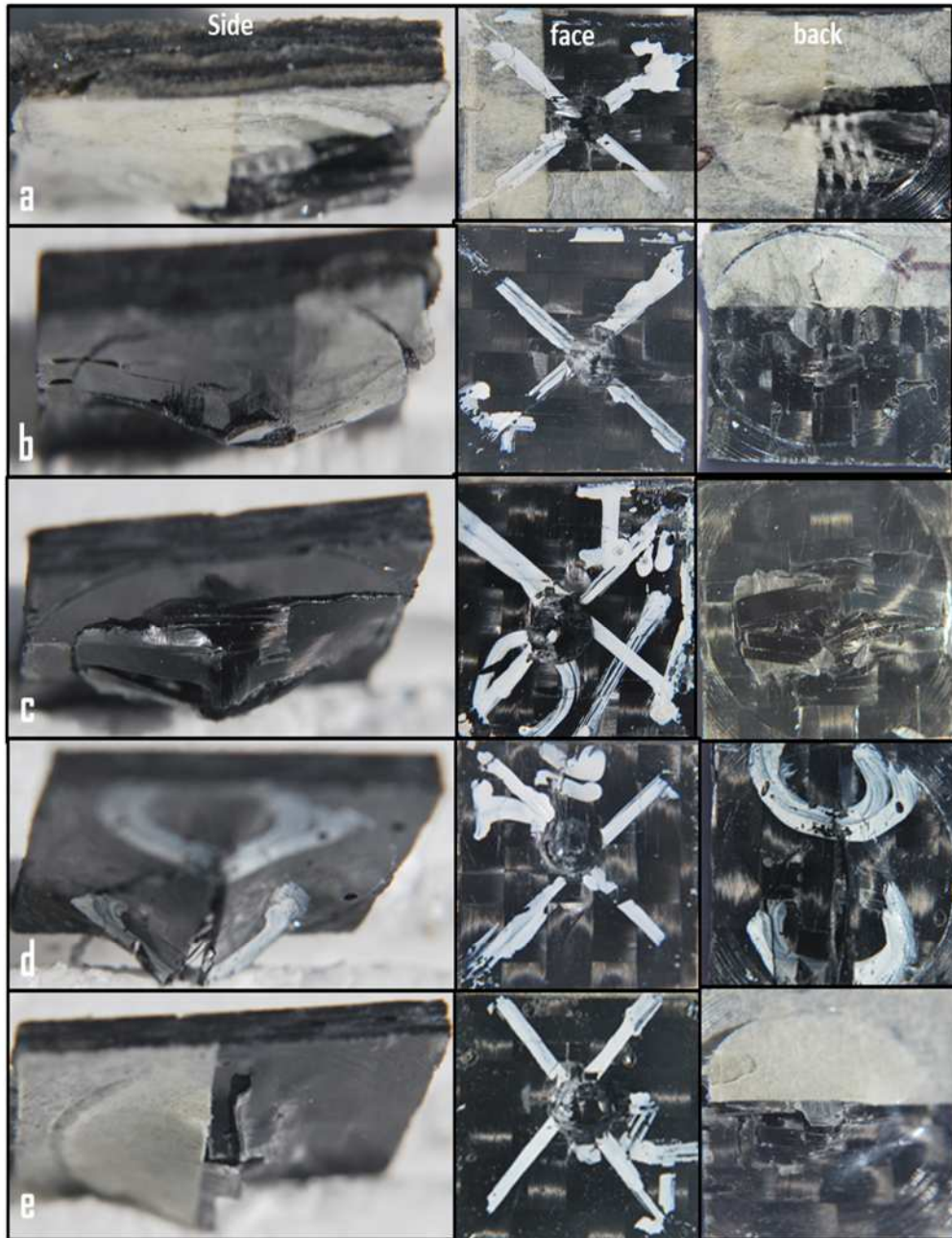
Figure 4.30: Optical image of specimen after damage resistance test for TPCL having differently oriented composites (skew angle)
