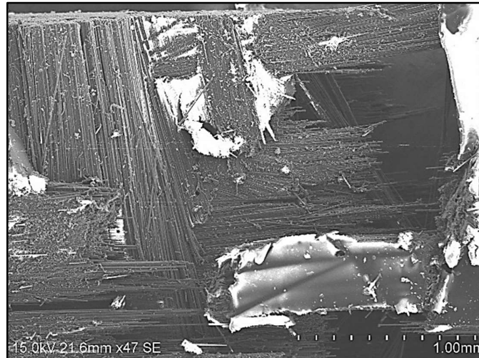
Figure 2: SEM images of tensile failure of sample with orientation angles as (0,90,90,0)
