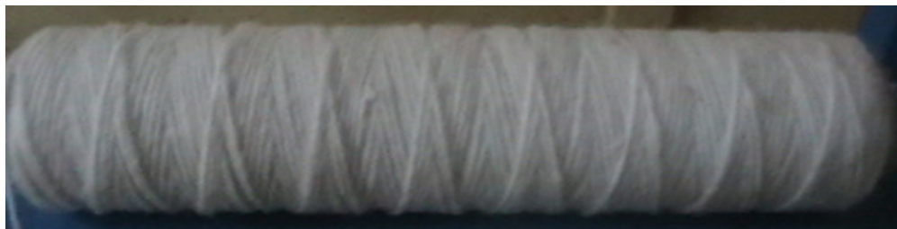
Fig. 3.24 shows a cartridge produced on newly developed winder ( 15^\circ /ATR=16.896)
