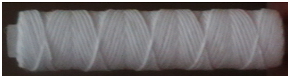
Fig. 3.25 shows a cartridge produced on fabricated winder ( 25^\circ /ATR=9.936)
