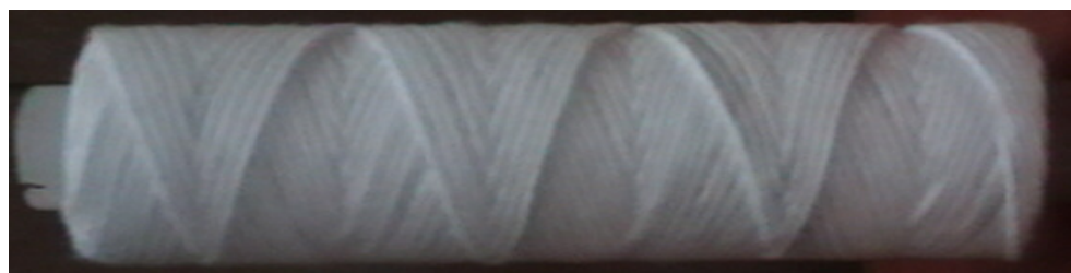
Fig. 3.26 shows a cartridge produced on fabricated winder ( 35^\circ /ATR=6.952)
