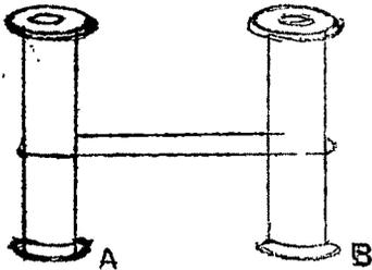
As the pulley 'A' rotates, the second pulley rotates in
