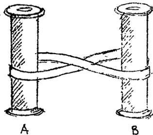
As the second pulley 'B' rotates in clockwise direction the first one
