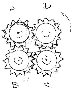
As the wheel 'D' rotates in the direction shown how do the wheels A and B move?
