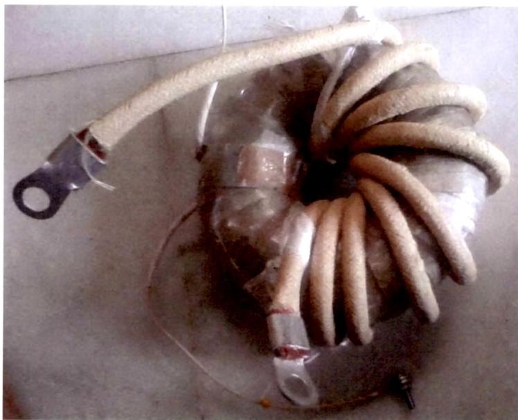
Figure 5.2: High Frequency Transformer
