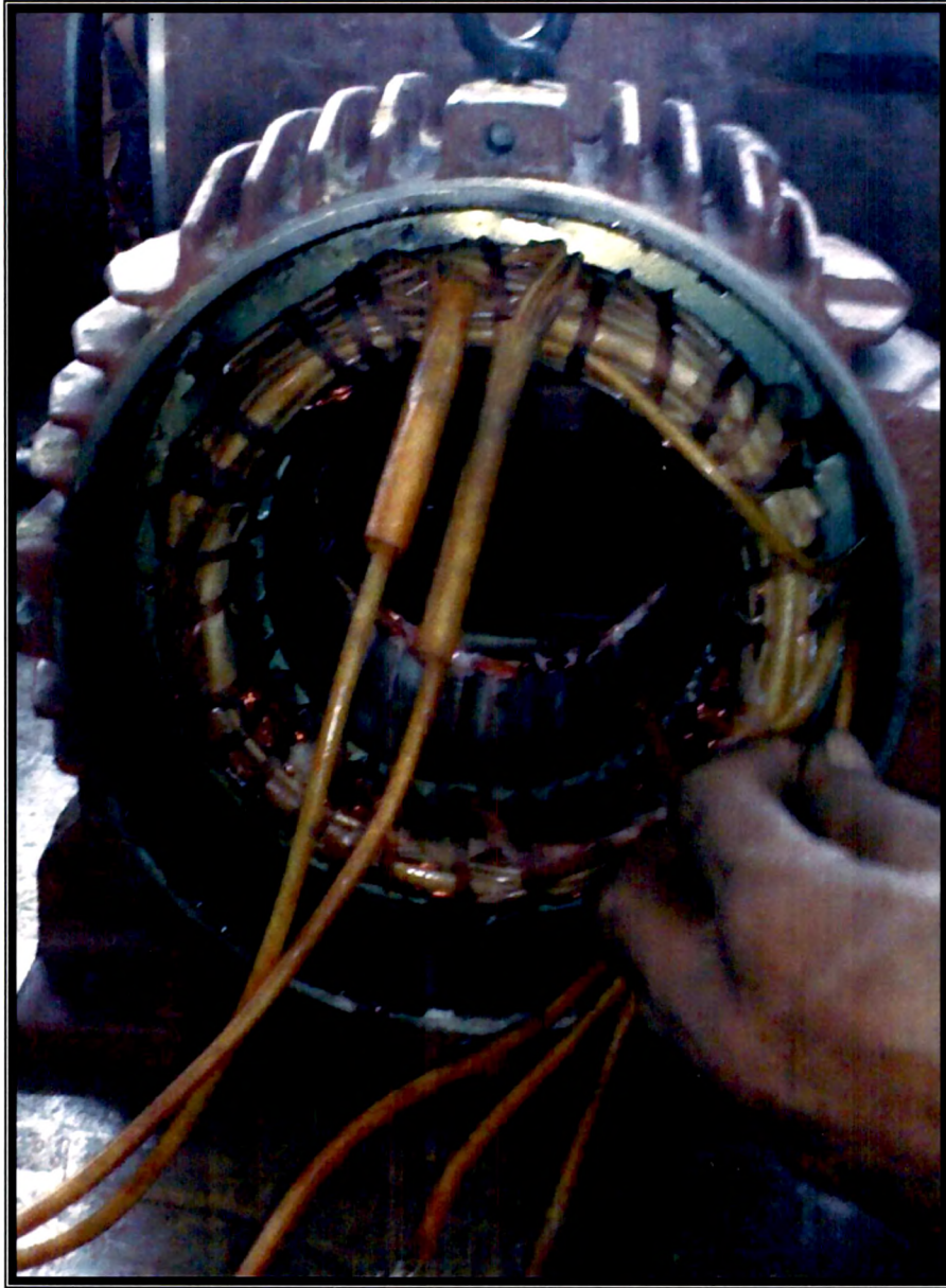
Photograph 3.2. Six phase stator after winding
