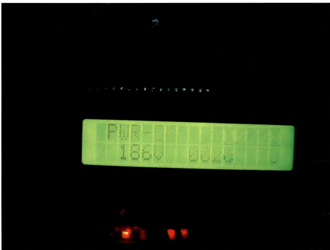
Figure B-5 LCD display of Mirco-controller Board (POWER-ON)
