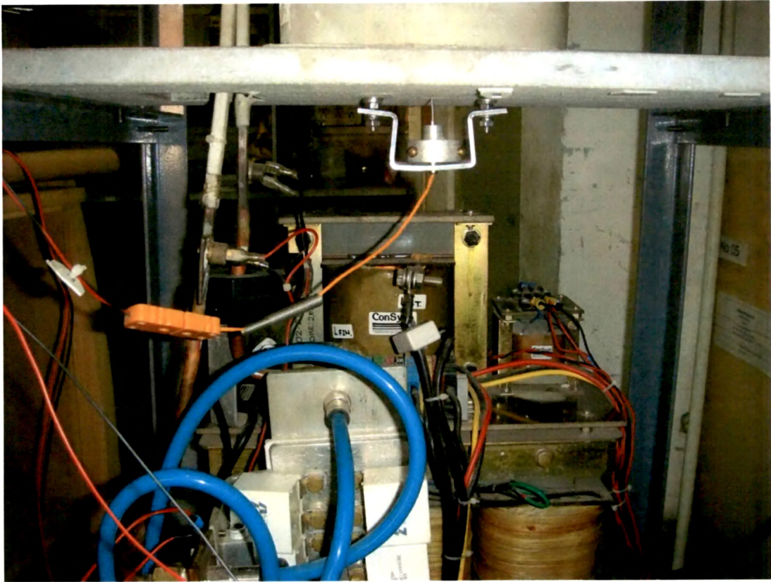
Figure B-2 Thermocouple Mounting
