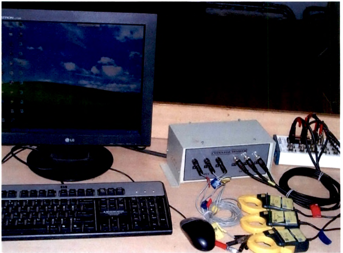
Photograph 5.1 Hardware for Motor Current Signature Analysis
