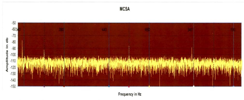
Figure 7.4: Current signature with Eccentricity fault
