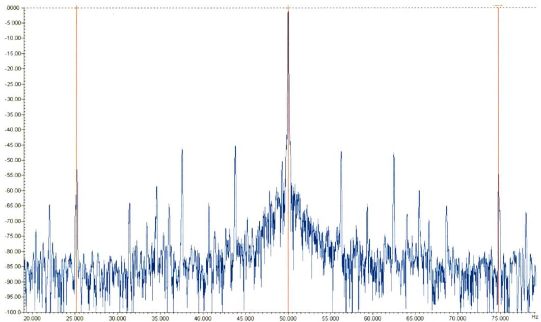
Figure 7.9: Current Signature with Torque Pulsation
