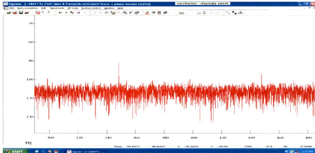
Figure 7.5: Current signature w/o Stator fault
