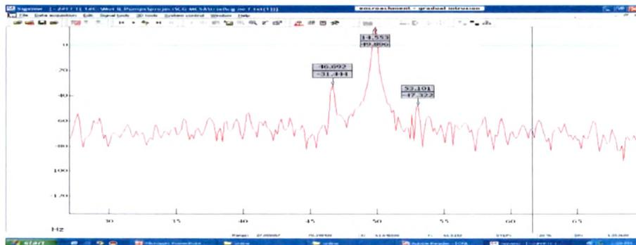
Figure 7.1: Current signature w/o rotor fault
