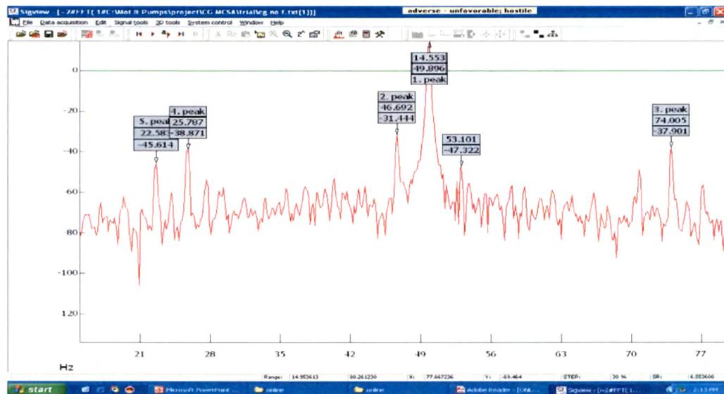
Figure 7.8: Current Signature with Misalignment between motor shaft and dynamometer
