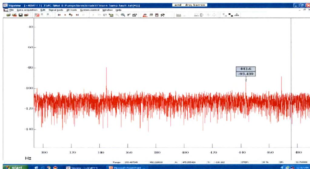
Figure 7.6: Current signature with stator fault- 15turn short
