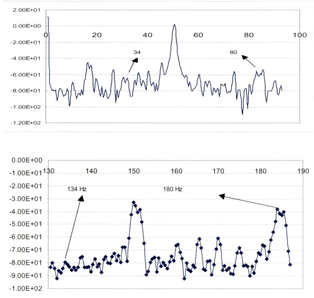
Figure 7.7: Current Signature in respective frequency bands with bearing fault-multiple fault on inner and outer race.
