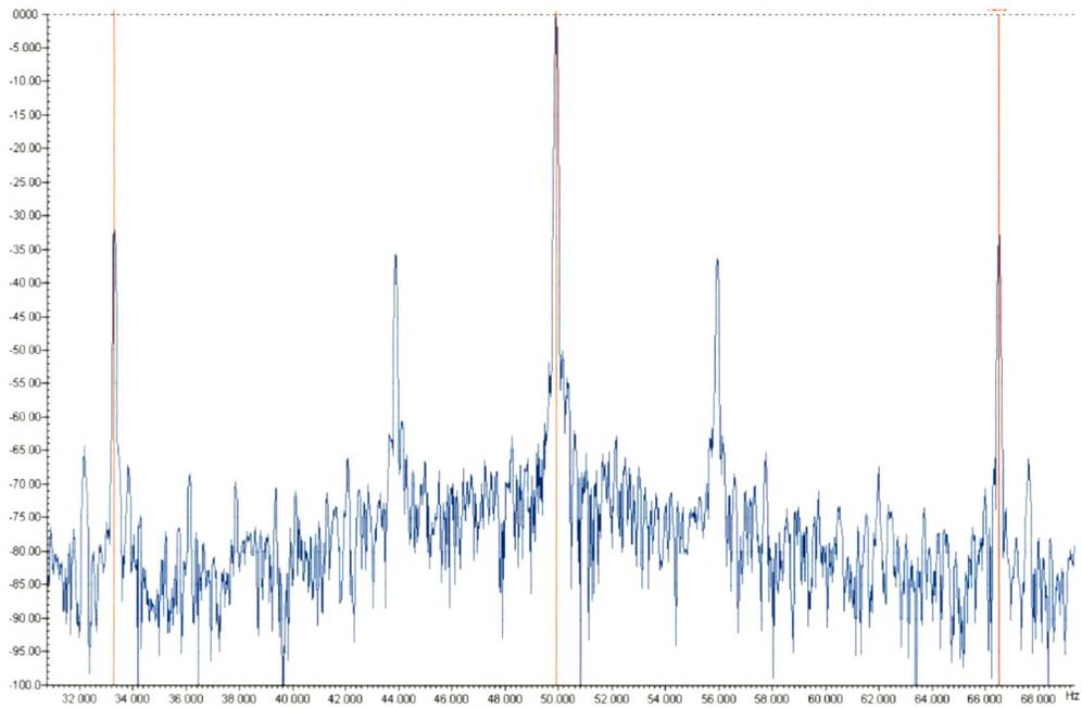
Figure 7.11: Current Signature with Rotor fault
