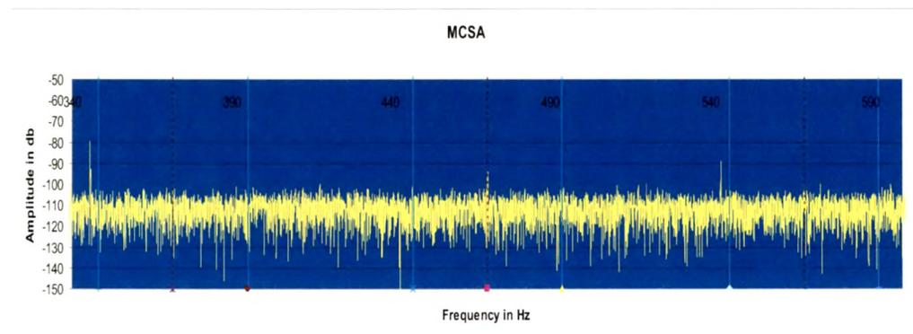
Figure 7.3: Current signature w/o Eccentricity fault
