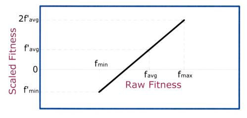
Fig. 4.2 Problems with Linear Scaling in Mature Run
