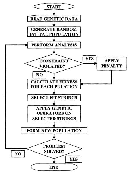
Fig 4.4 Flowchart of GA based Optimization Procedure
