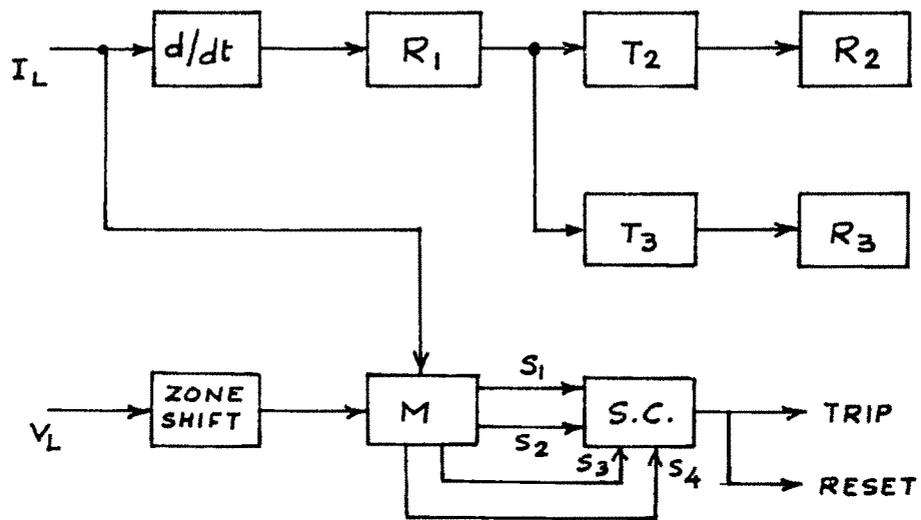
FIG. 4.9 BLOCK-SCHEMATIC DIAGRAM OF THE 3-STEP RELAY
