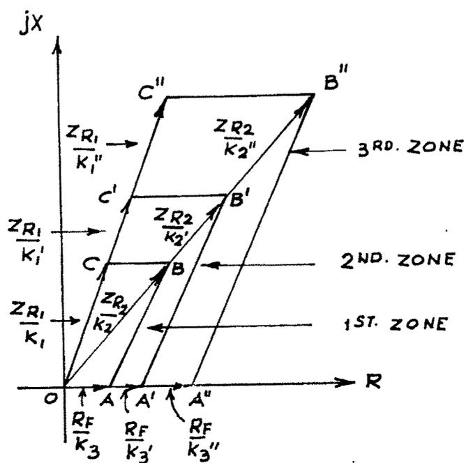
FIG. 4-8 3-STEP QUADRILATERAL CHARACTERISTICS
