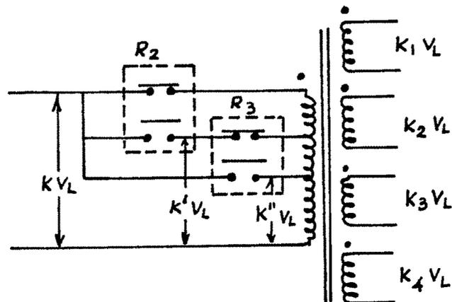
FIG. 4-10 CONTACT ARRANGEMENT FOR ZONE SHIFTING.
