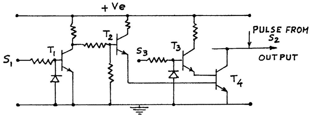
FIG. 4.4 3-INPUT SEQUENCE DETECTOR
