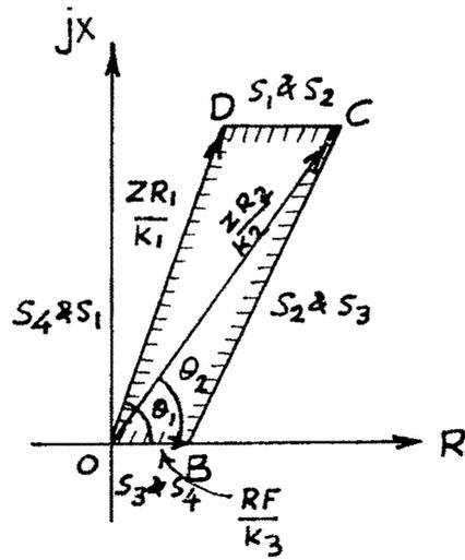
FIG. 4.3 QUADRILATERAL CHARACTERISTIC
