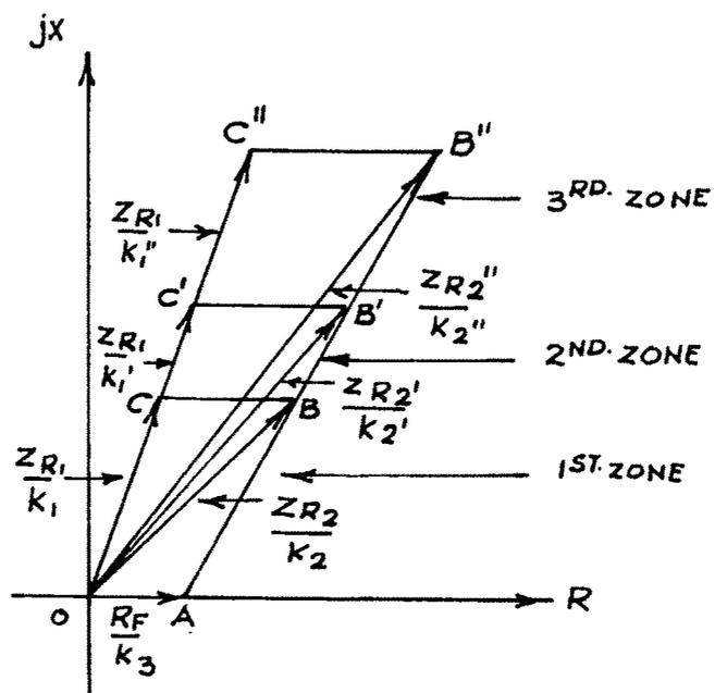
FIG. 4.11 3-STEP QUADRILATERAL CHARACTERISTICS
