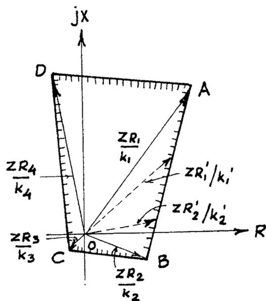
FIG. 4.1 QUADRILATERAL CHARACTERISTIC
