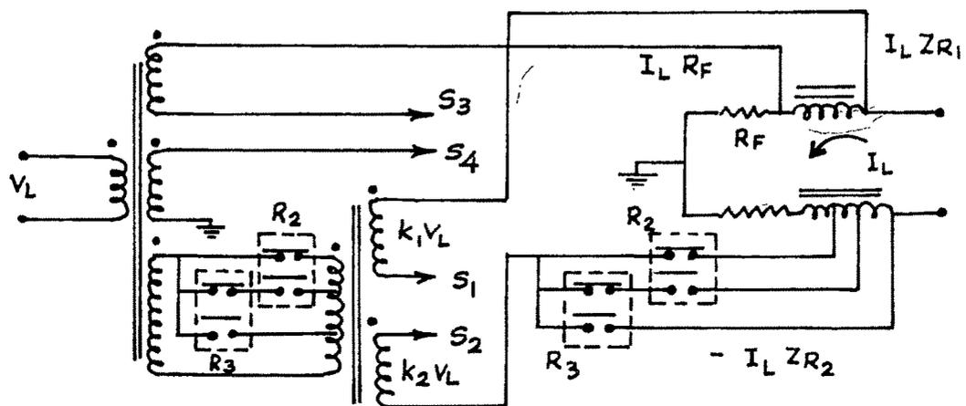
FIG. 4-12 MEASURING CIRCUIT WITH CONTACT ARRANGEMENT
