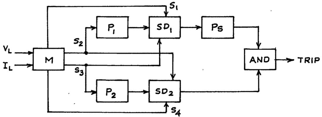
FIG. 4.6 BLOCK-SCHEMATIC DIAGRAM OF THE FIRST ZONE RELAY
